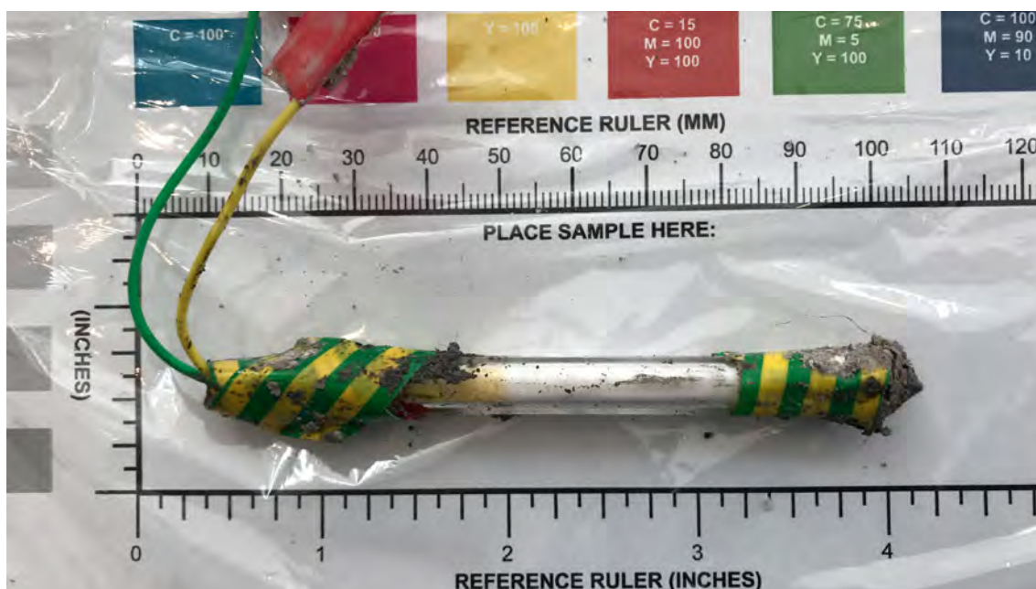
Image 189. Electrically initiated detonator using improvised chlorate and organic peroxide explosives (source: BCL ©)
