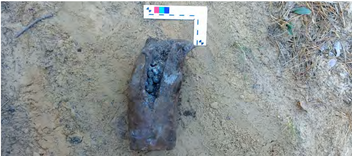
Image 115. Aged artillery shell with anti-personnel effect in sandy soil. The shell was exposed to an explosion 65 years prior to its finding. The greyish-yellow TNT filler, exposed to the environment, is partly visible amongst the fragmentation balls (source: GICHD ©)
