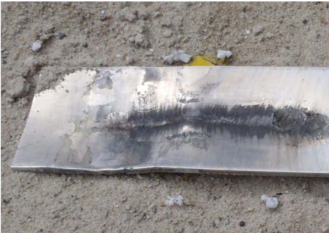
Image 15. The effects of an improvised detonator (filler: TATP) on an aluminium witness plate (source: BCL ©)
