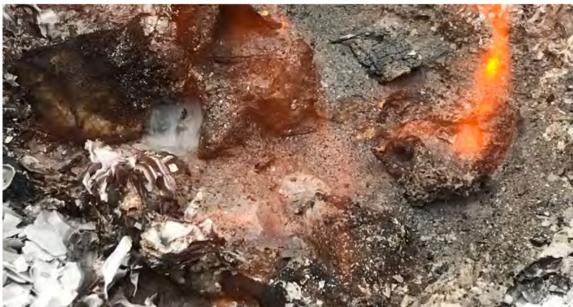
Image 179. Remains of an improvised incendiary (gel-based), which has reignited when exposed to atmospheric oxygen in the disturbed ashes of a commercial property (source: BCL ©)
