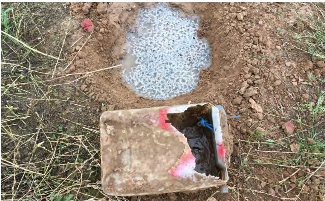
Image 117. Effects of ageing: aluminium powder after separation from ammonium nitrate (source: FSD ©)
