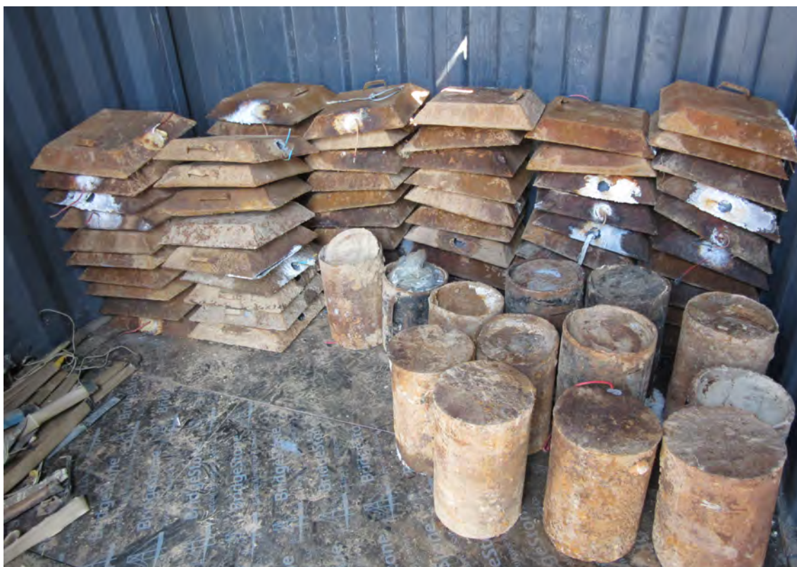
Image 5. Example of different main charges filled with HME (source: Fondation Suisse de Déminage FSD ©)
