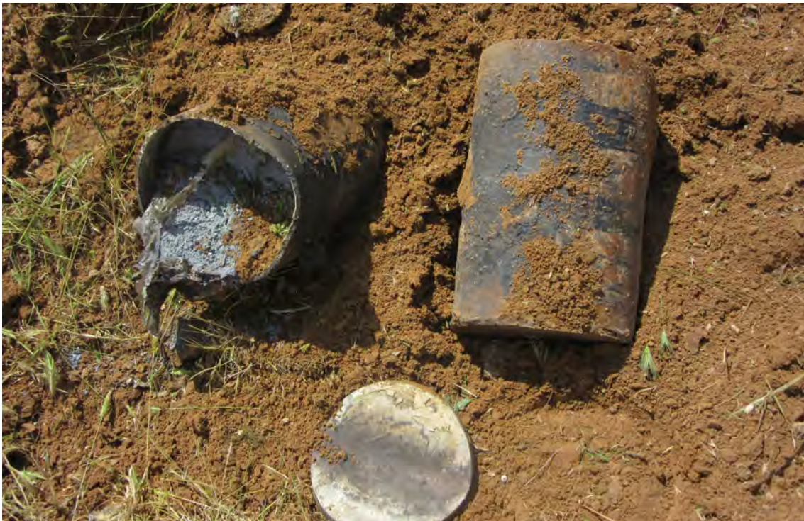
Image 6. Main charges filled with HME of unknown quality and sensitivity posing explosive and non-explosive hazards (source: FSD ©)
