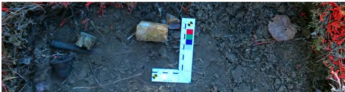
Image 2. Example of an explosive homogeneous compound: TNT (here used as filler for artillery shells) (source: GICHD ©)
