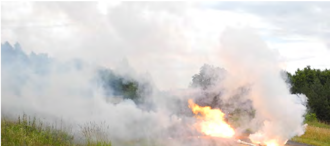
Image 18. Example of the burning behaviour of solid propellants when unconfined (source: GICHD ©)
