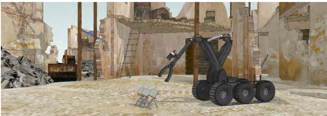
Image 6. ROV remotely placing a shaped charge array to target a buried IED
