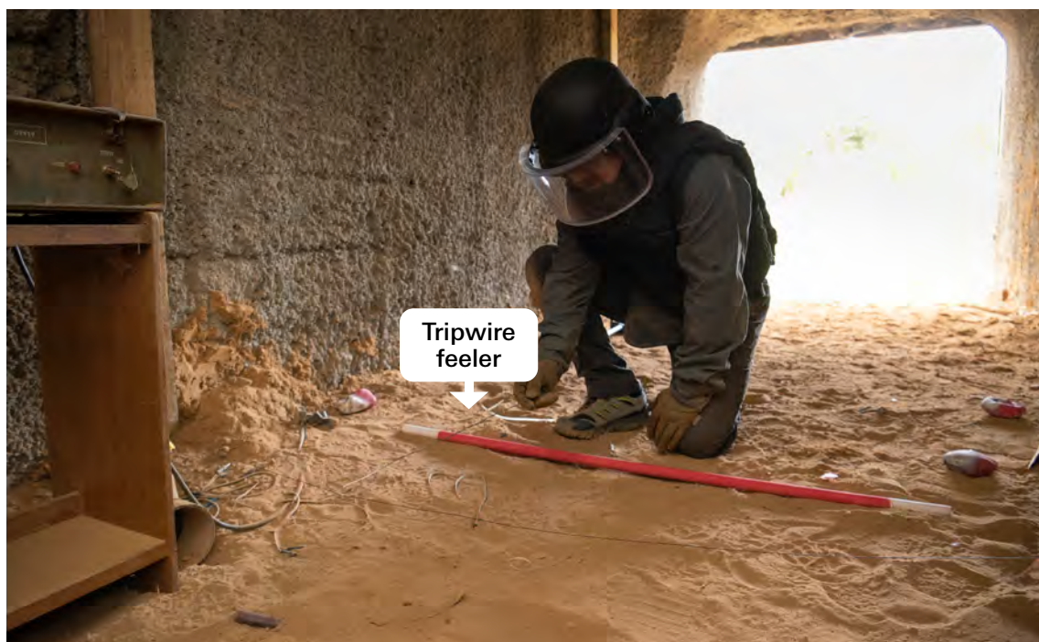
Image 9. Using a tripwire feeler in a passageway where there is less natural light
