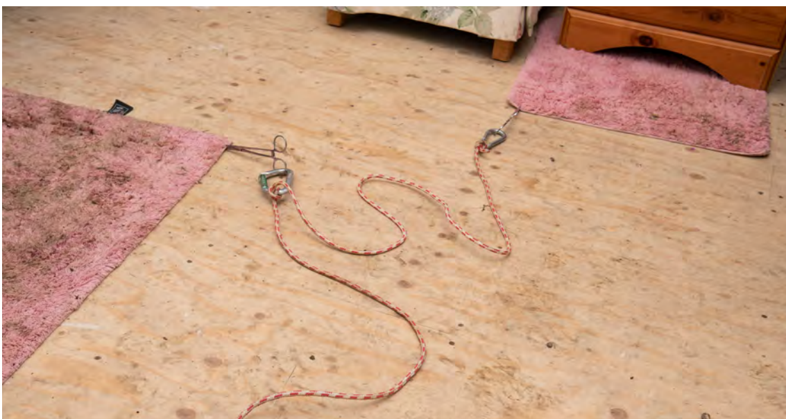
Image 13. A typical semi-remote search set-up in buildings and structures arranged for pulling multiple items on one pull
