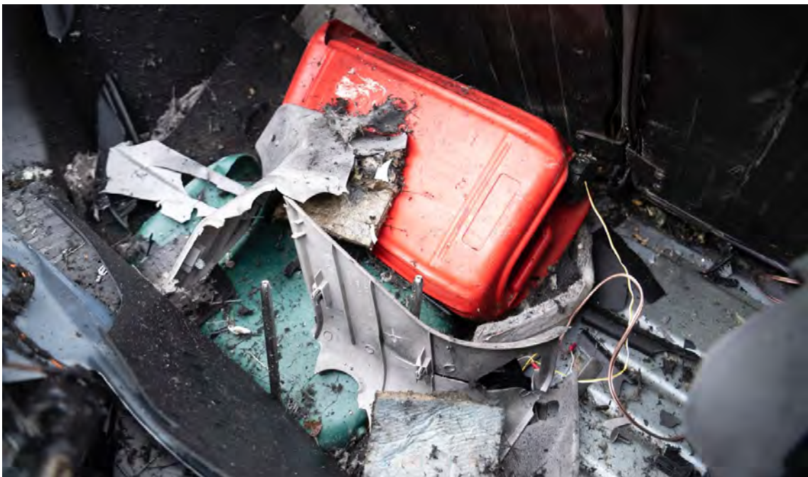
Image 17. Main charges in the trunk post disruption. Note how the seats have shielded this area and prevented disruption of any items in the trunk
