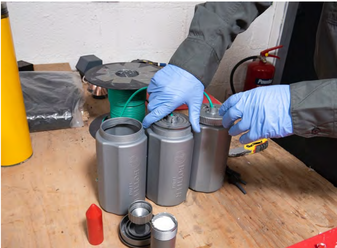
Image 3. Inserting the inner chamber and securing the lid on a commercial bottle disruptor. Water will be added prior to use
