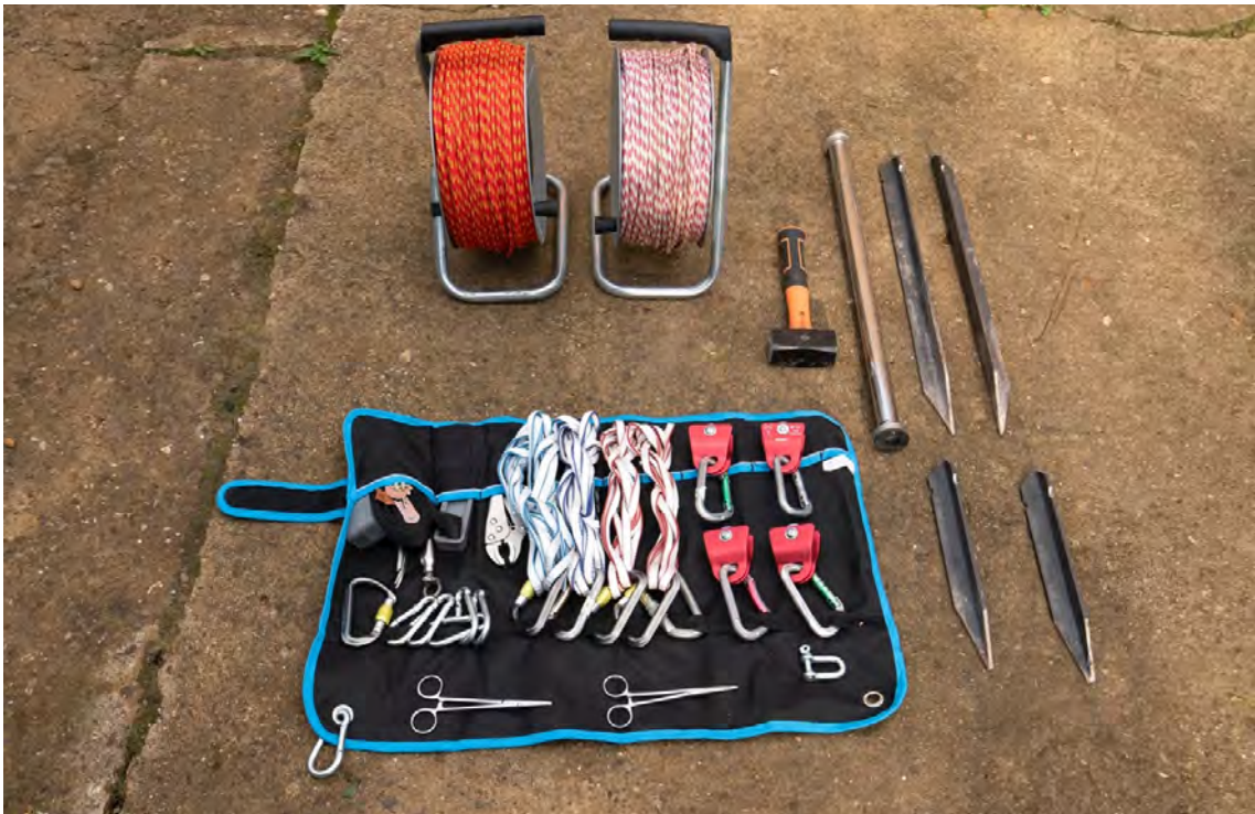
Image 1. Locally produced H&L kit. Individual items have been locally purchased to build an overall kit. Note how the items are of good quality / reliability to prevent unnecessary failures / breakages
