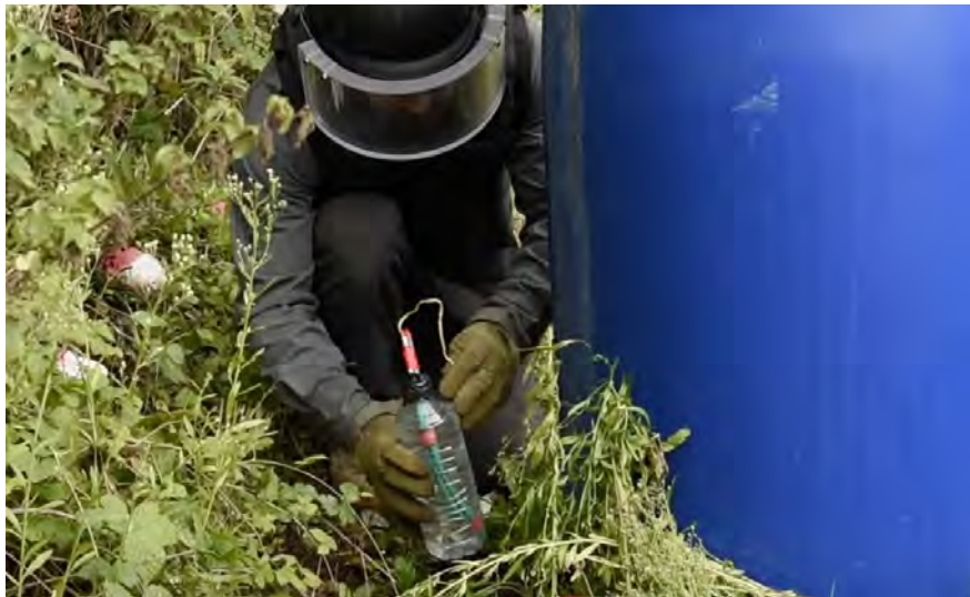
Image 4. IEDD operator placing a bottle disruptor
