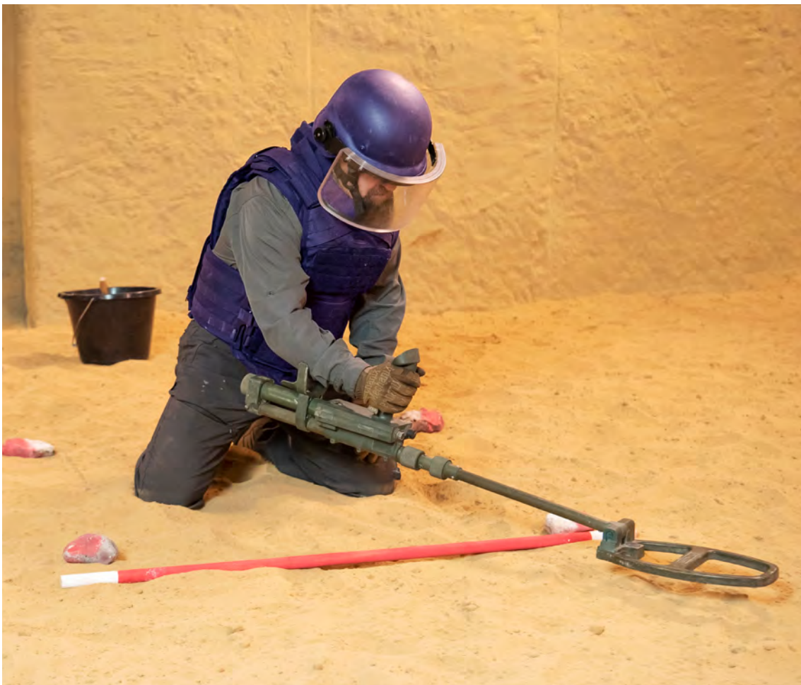
Image 3. Using the detector from inside the safe area using a stable kneeling position
