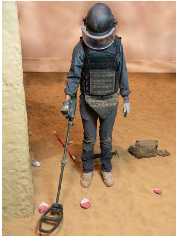
Image 15. The primary metal detector used to search other likely main charge locations
