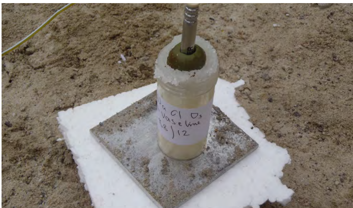
Image 133. Sodium chlorate–petroleum jelly, demonstrating the identical appearance to that of potassium perchlorate–petroleum jelly (source: BCL ©)
