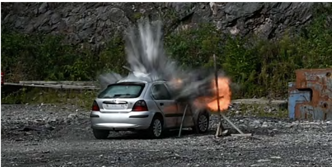
Image 21. Improvised VBIED disruptor functions. Note the flash from the detonating cord but the water has largely suppressed the bulk explosive in the disruptor HD version from video required
