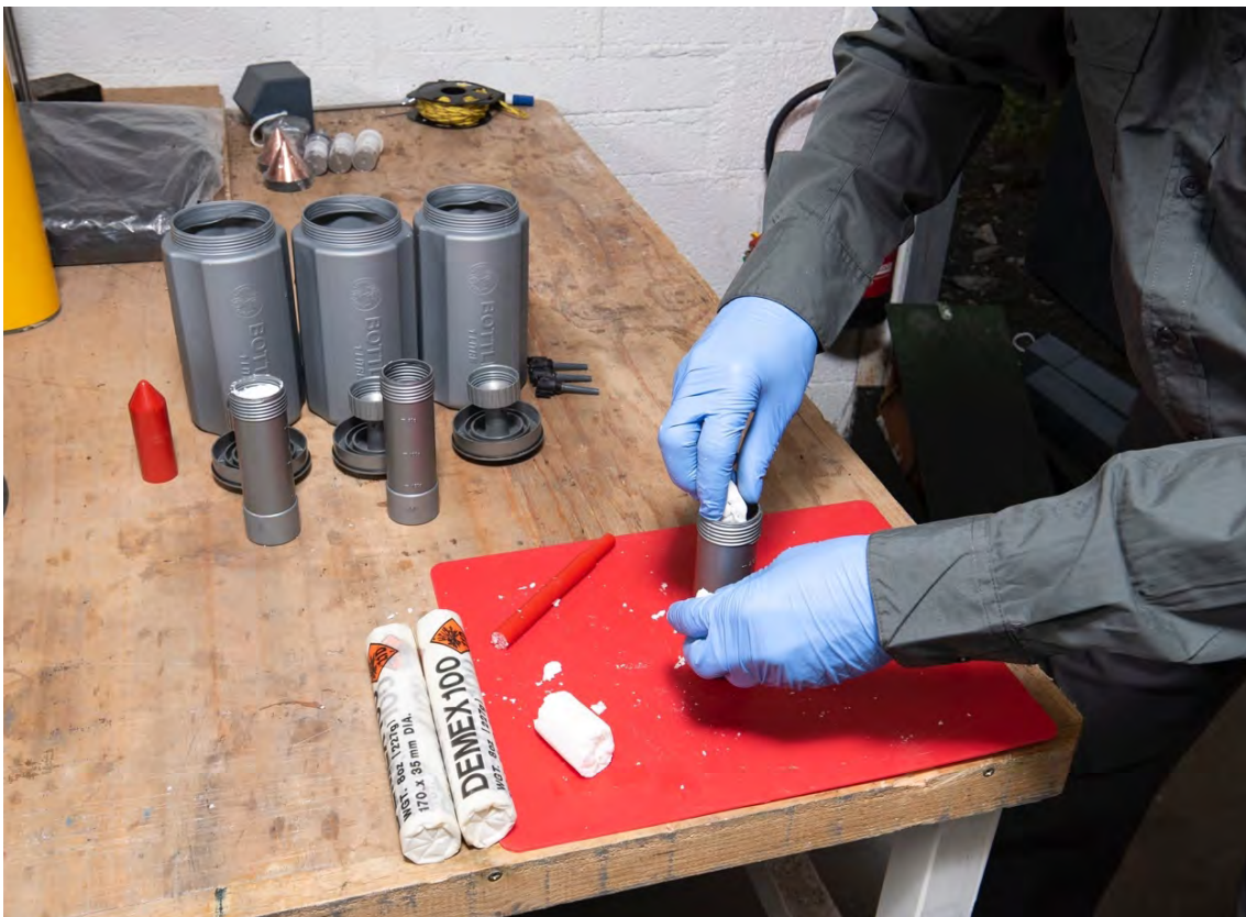
Image 1. Loading plastic explosives into the inner chamber of a commercial bottle disruptor
