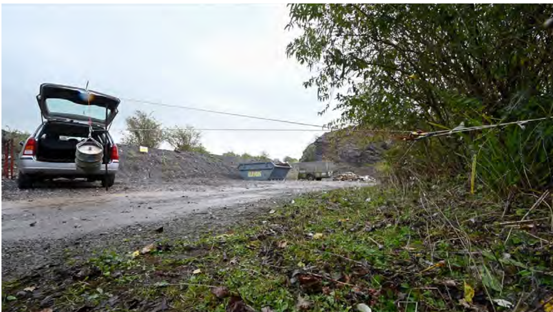
Image 13. The red line is used to lift the main charge then the white line is used to pull the main charge clear of the vehicle
