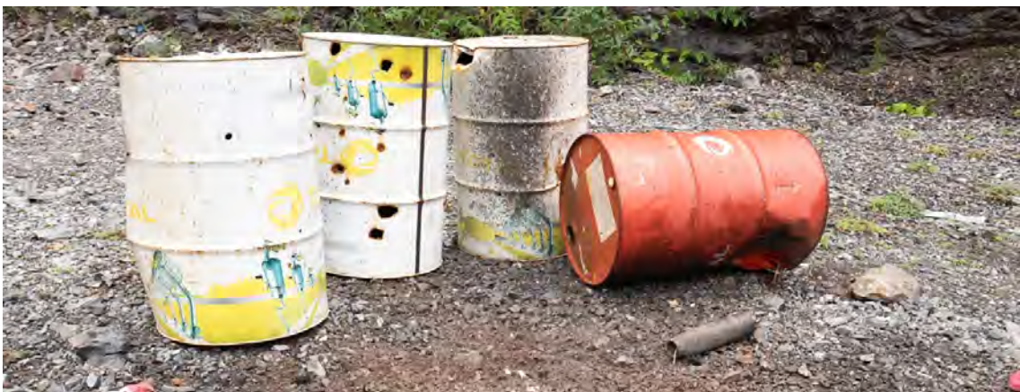
Image 9. Effect post disruption. Note how the projectile and oil drum have also been moved by the force of the bottle disruptor
