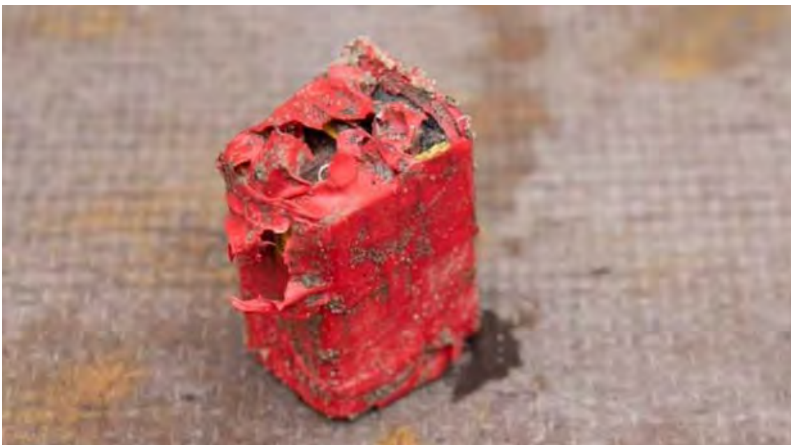
Image 15. Power source post disruption. Note how the power source is intact and just the leads have been removed
