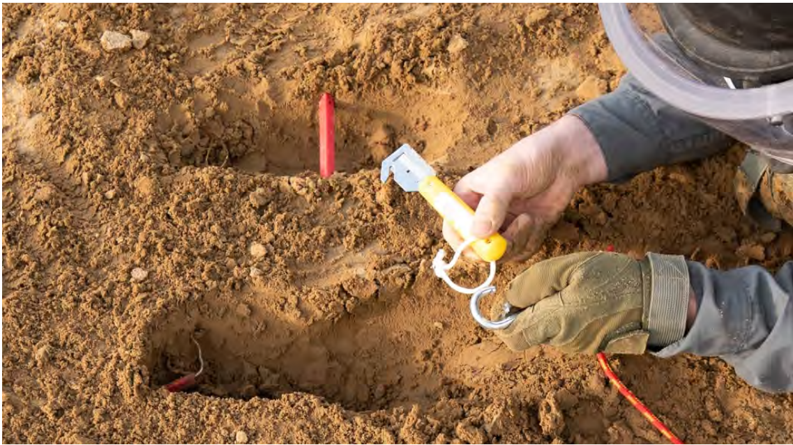
Image 2. Preparing an H&L cutter. Here the IEDD operator has opted to attach the line before placement as they have assessed this to be a better course of action in this situation
