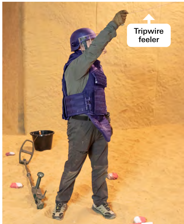
Image 8. Increase the height of the tripwire feeler as high as the operational threat assessment dictates
