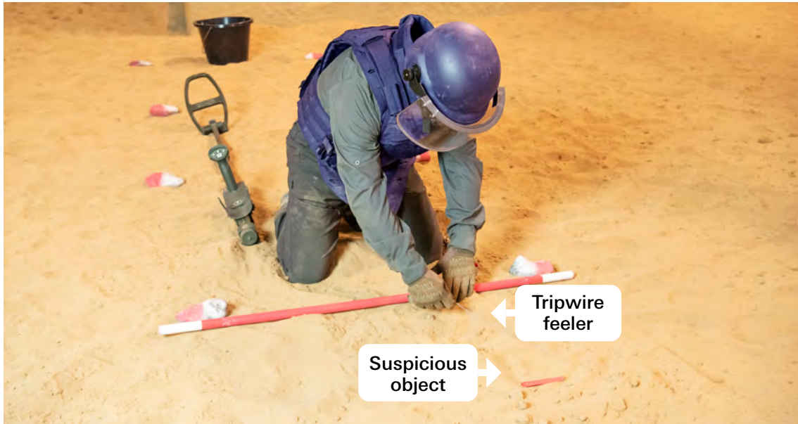
Image 2. Tripwire feeler being laid on searched ground pointing to the object for handing over to an IEDD operator
