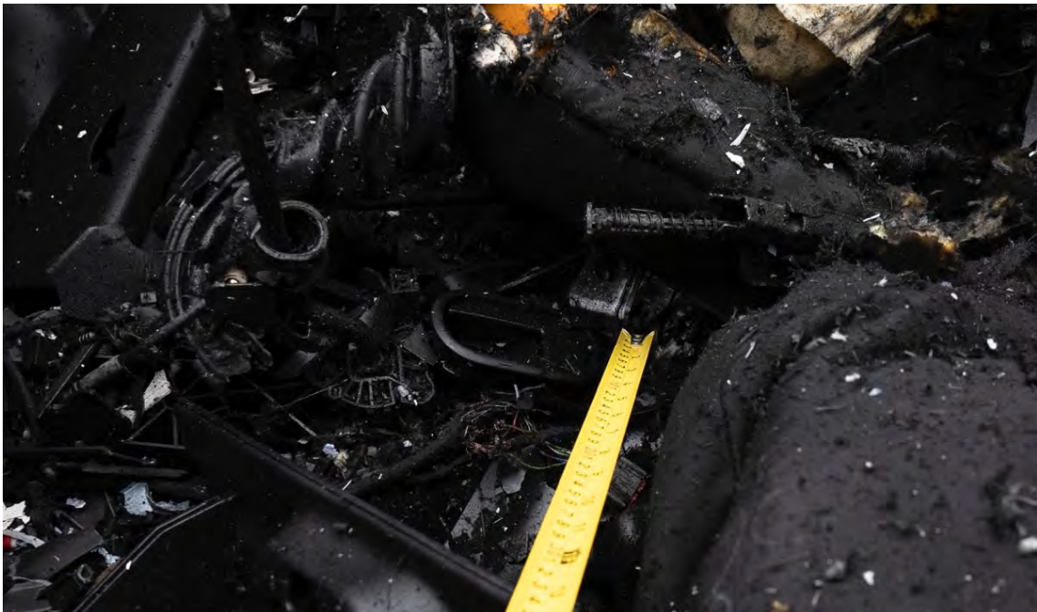
Image 16. Tape measure points to the battery from the mobile telephone close to the original location of the RC pack
