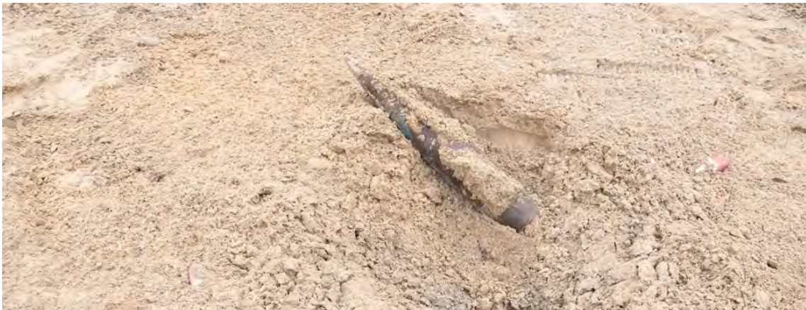
Image 5. The effect post disruption. Note how the 155 mm projectile has also been moved by the force of the bottle disruptor
