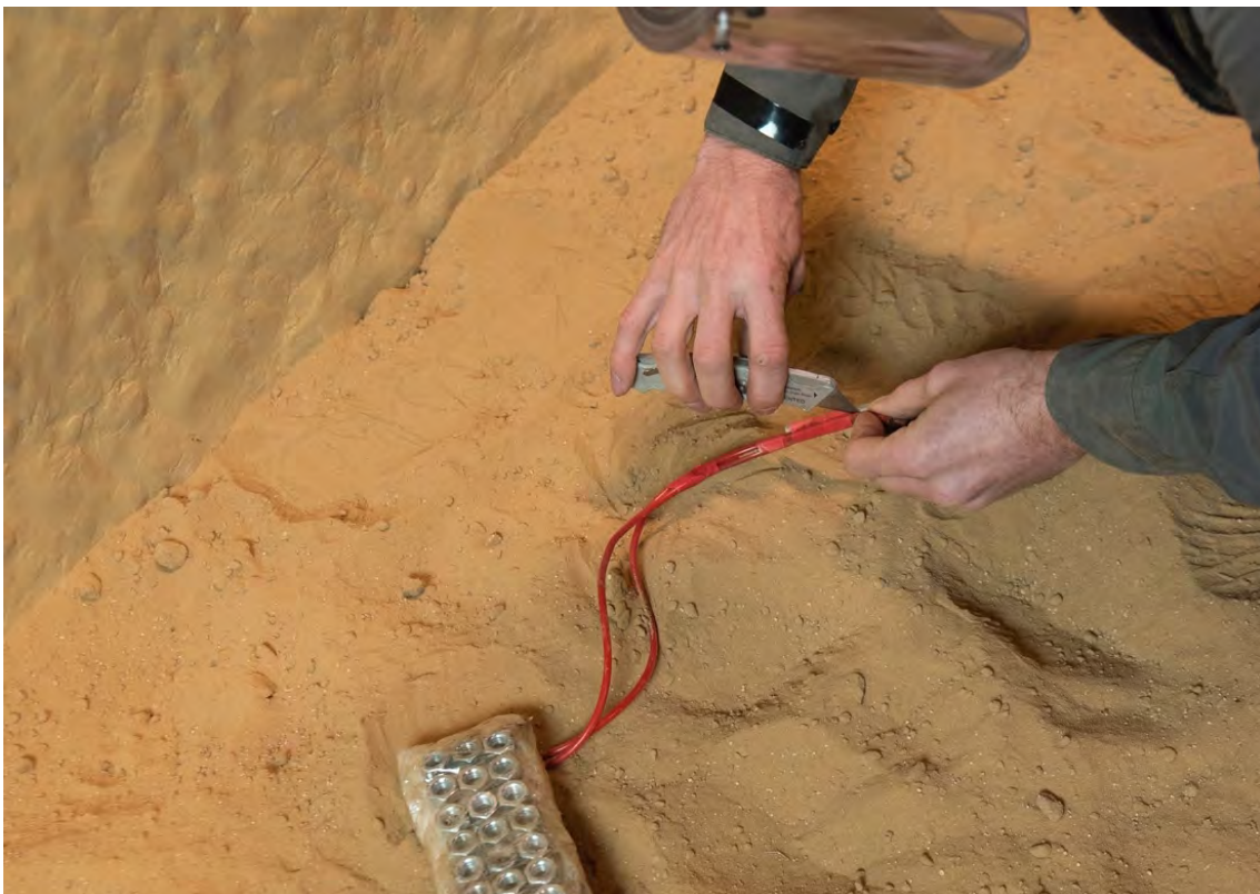
Image 4. Sharp knife or scalpel used to cut one side of the PAT holding the detonator to the detonating cord. Note: the IEDD operator is cutting away from themselves to avoid injury
