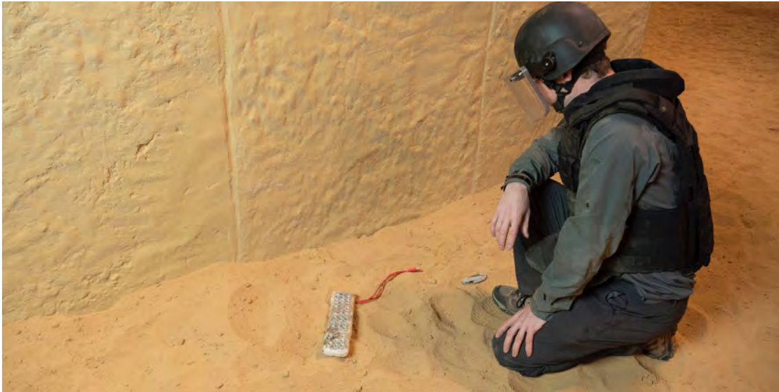
Image 1. Main charge of a suicide belt with an electric detonator attached to the detonating cord. All other IED components have already been removed as part of the RSP
