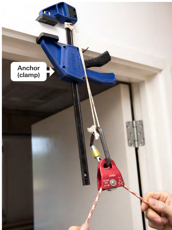
Image 9. An off-the-shelf clamp used as an anchor for changes of direction with white prusik cord loop, karabiner and pulley
