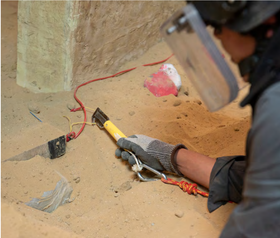
Image 14. Placing a J Knife cutter to semi-remotely sever an electrical wire. This technique may become the primary option when access to energetics is restricted
