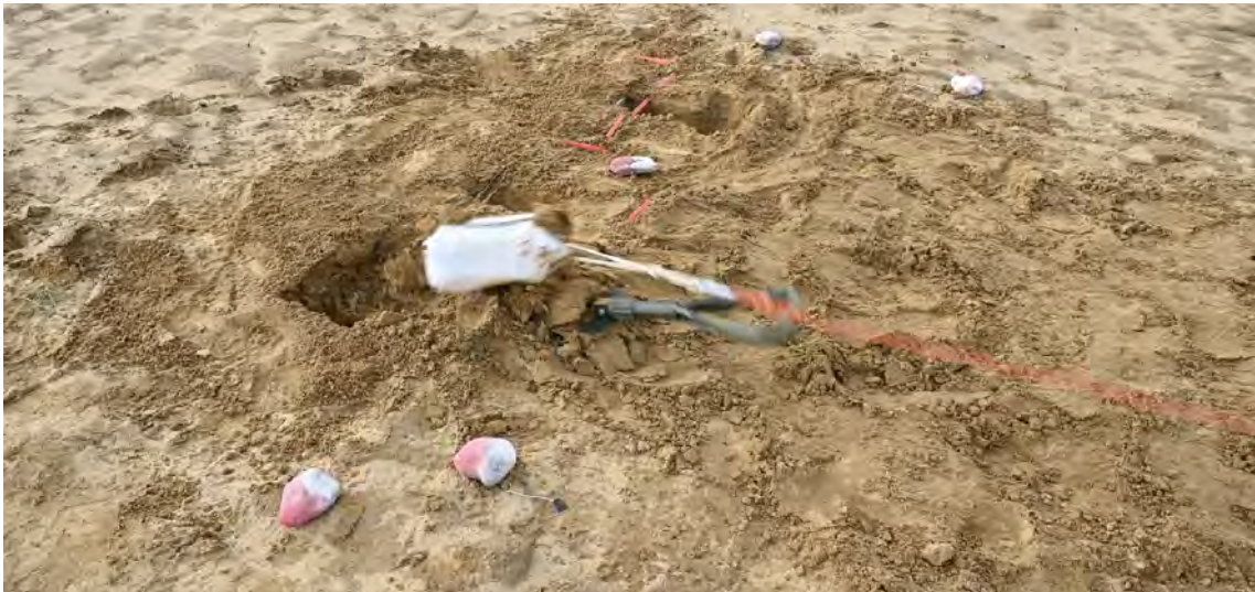
Image 10. Using the spade to create an elevated pivot point aids in removing the main charge by lifting and pulling it
