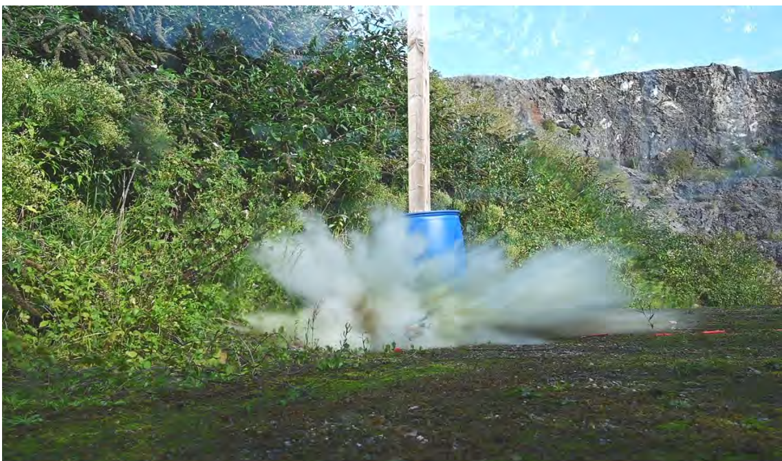
Image 21. Improvised 500 ml bottle disruptor functions and the water suppresses the heat and flash
