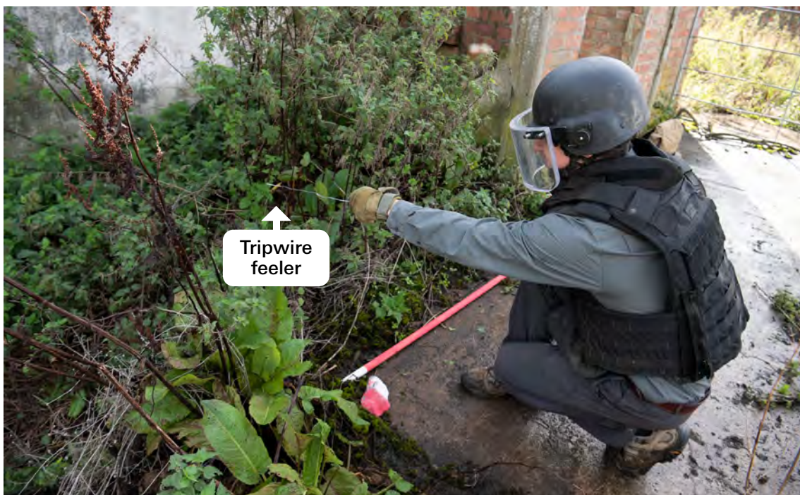
Image 2. Use of a tripwire feeler as an aid to visual search in the top layer of vegetation
