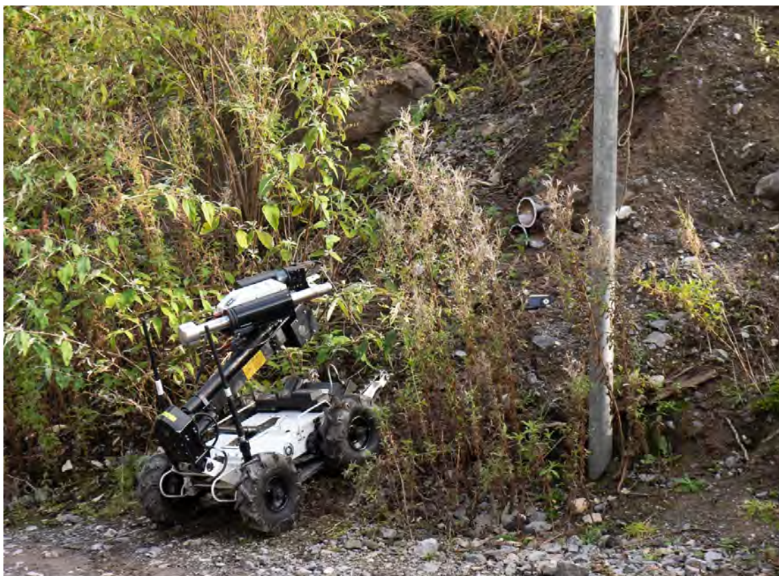
Image 2. ROV conducting EOR of an EFP array placed at the roadside
