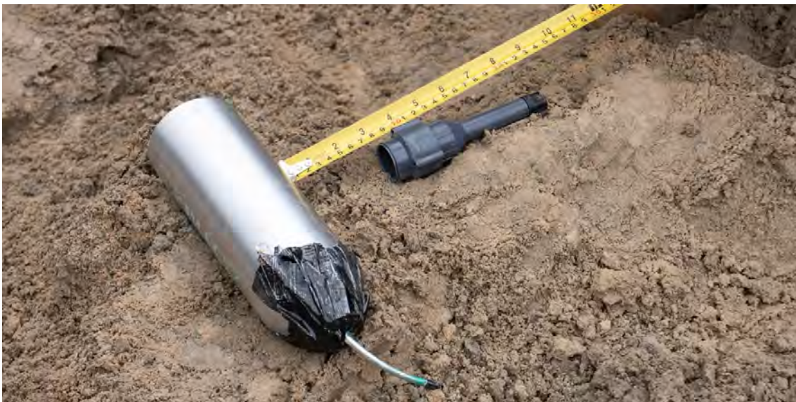
Image 8. Shaped charge with magnesium jet forming cone, filled with 50 g of high explosives (DEMEX) placed with 75 mm stand-off from an abandoned IED main charge
