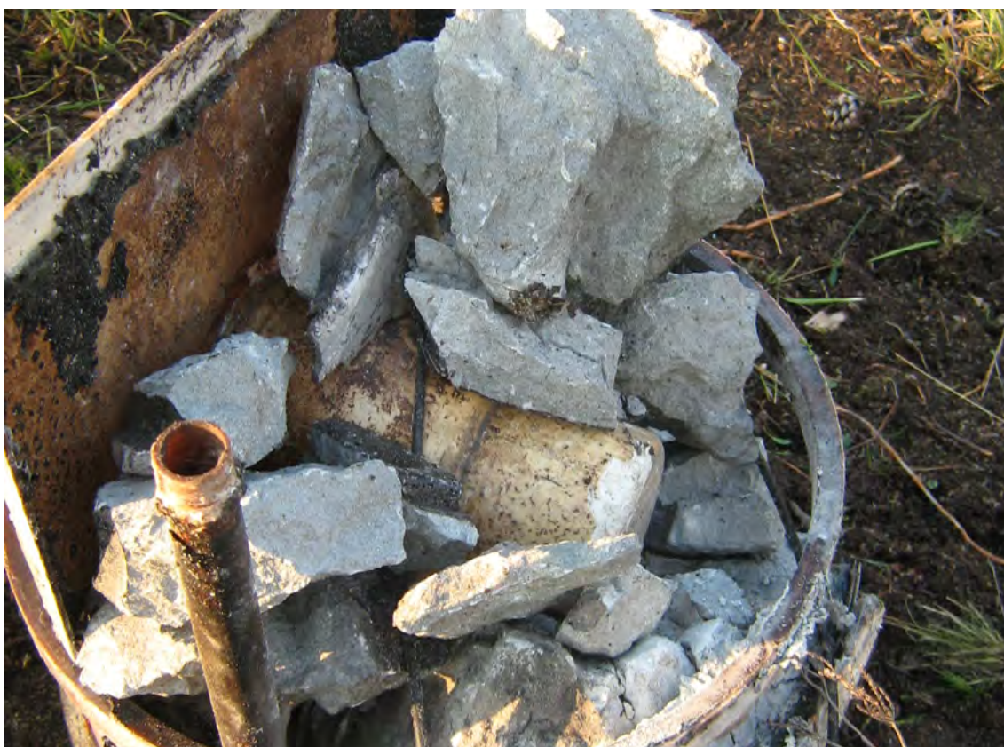
Image 4. Example of a military explosive: remnants of a torpedo warhead filled with Torpex (RDX, TNT, aluminium powder and wax) (source: GICHD ©)
