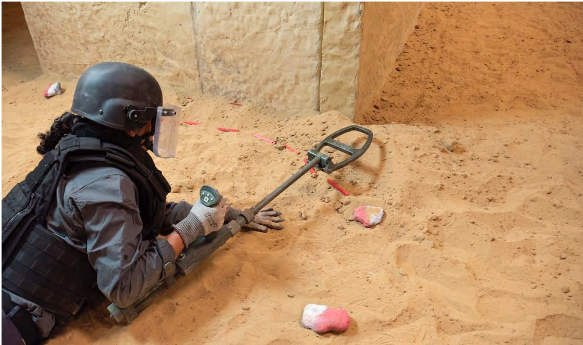
Image 9. Metal detector used in prone position
