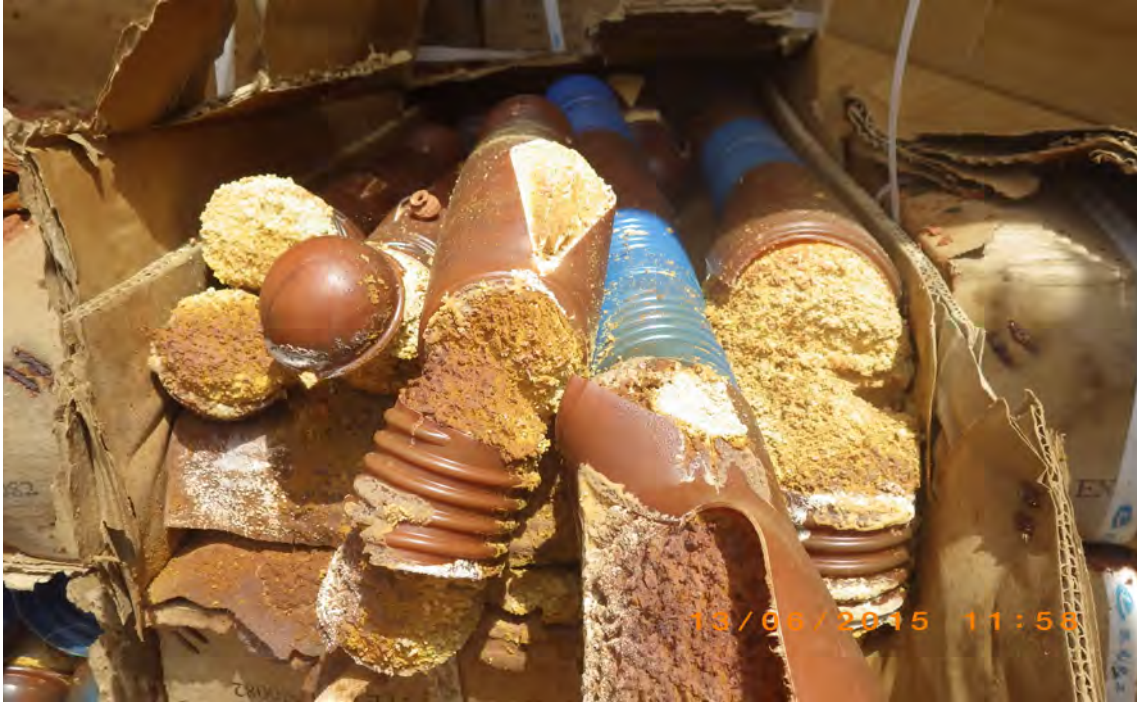
Image 118. Ageing: unknown mining explosive aged after being stored in a non-air-conditioned container in a tropical location for an unknown time. The casing is destroyed and discoloration of the explosive is recognisable. The chemical effects of ageing on the explosive cannot be estimated (source: Stanislav Damjanovic ©)
