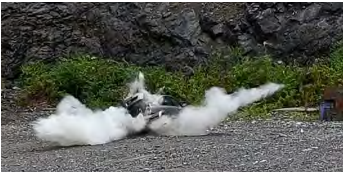
Image 32. Note how much the water has suppressed the flash from the detonation. This reduces the risk of a vehicle fire
