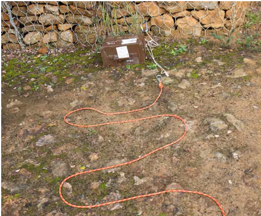
Image 1. H&L prepared and awaiting attachment of the main line on a strop. Note the prepared slack in the main line and a tether secured to a hard point to cause the container to open
