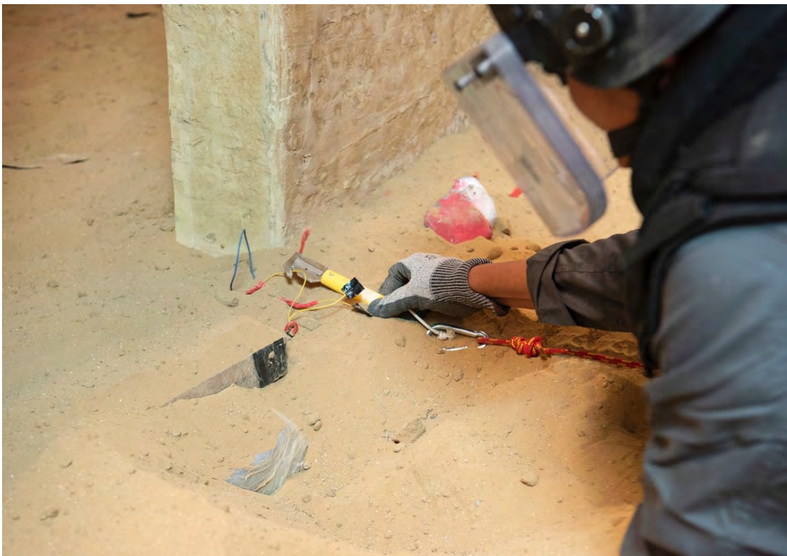
Image 22. Placing semi-remote cutter against second detonator lead. (Red cable is a strop)
