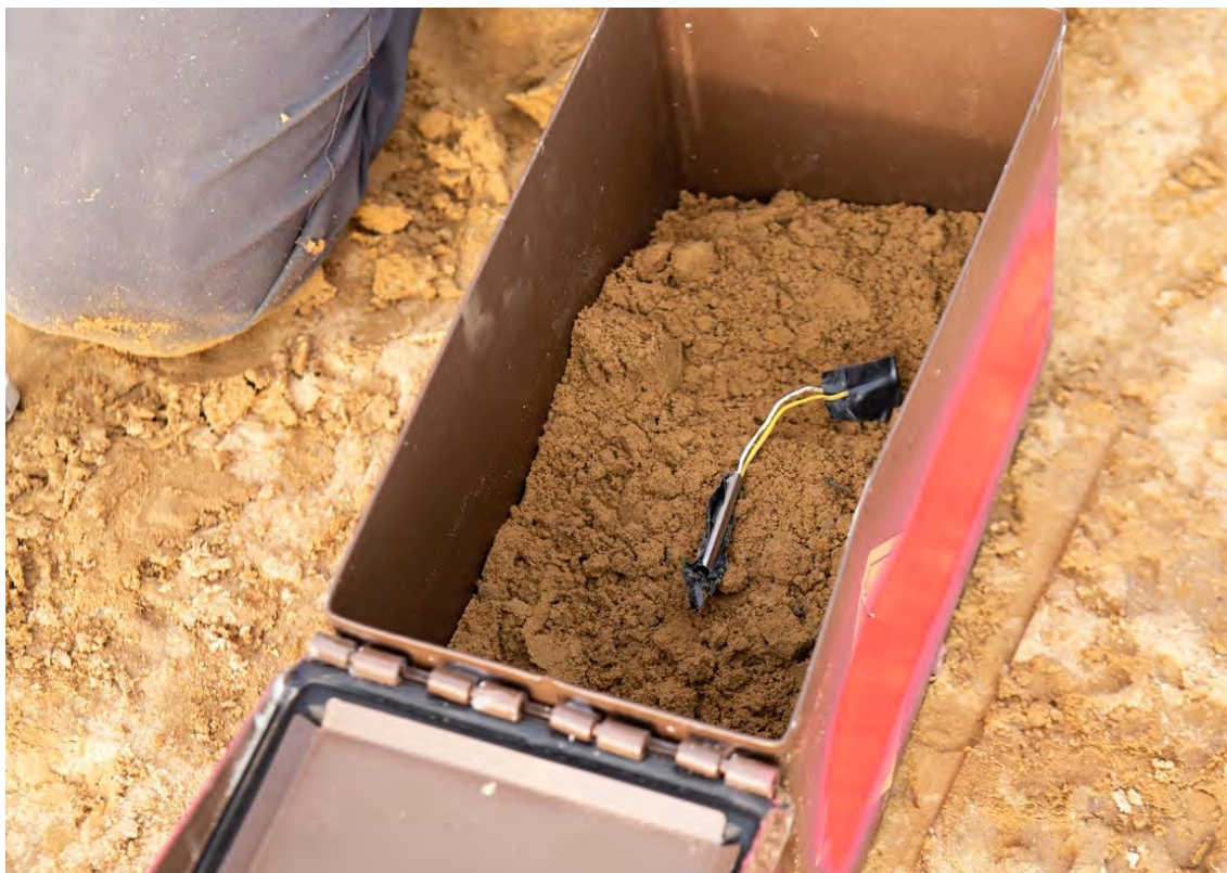
Image 7. Detonator placed in a rigid metal box to screen from RF and protect from damage
