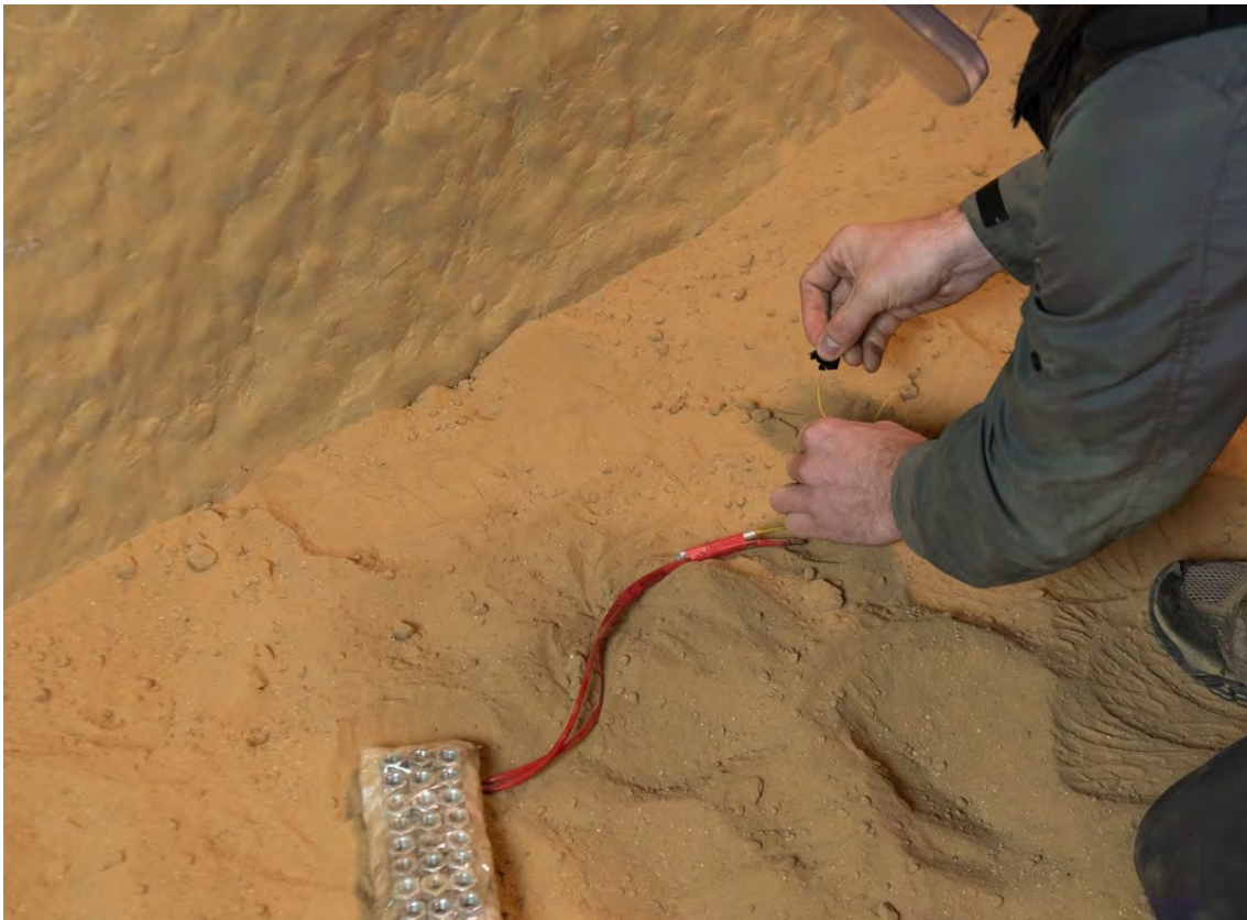
Image 2. Insulation tape used to insulate leads from static
