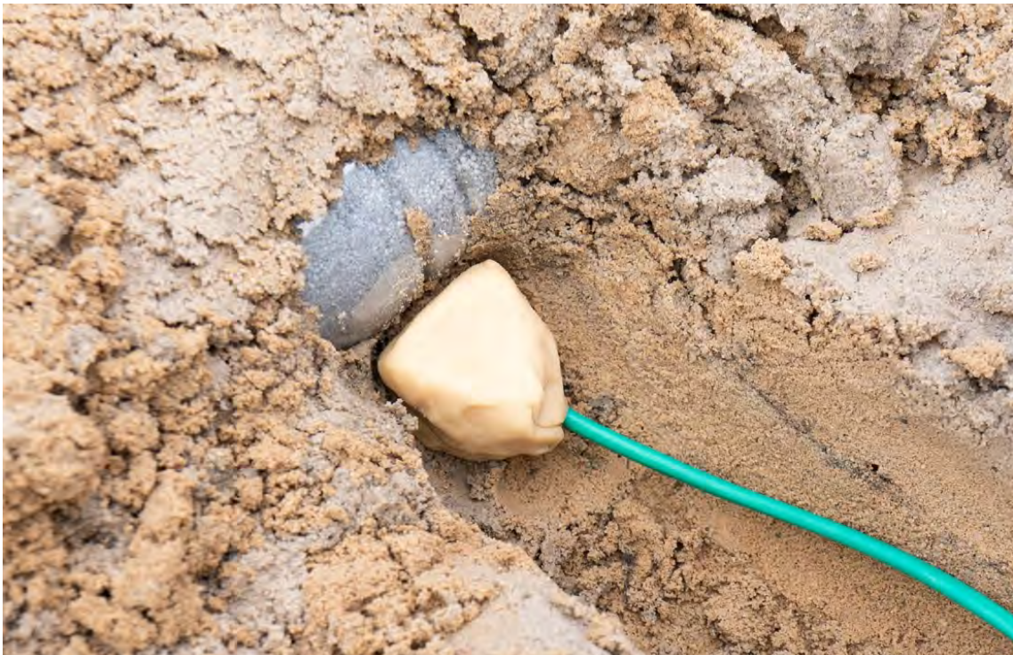
Image 3. Donor charge placed in the channel as close to but not touching the IED main charge
