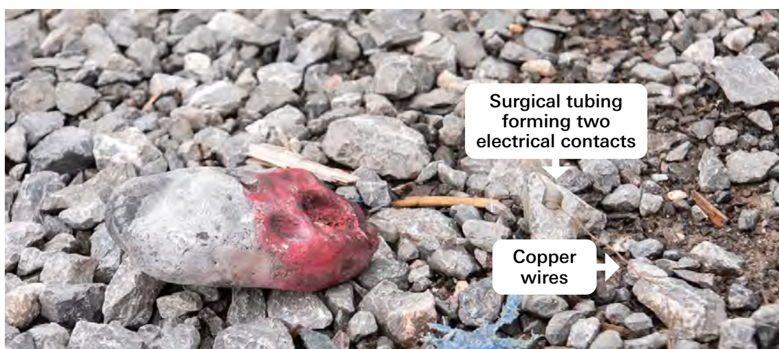
Image 6. Example of a crush wire switch. Note: these two copper wires would be covered with a lacquer insulation, which is removed at the point where it is wrapped around the surgical tubing in order to form two electrical contacts
