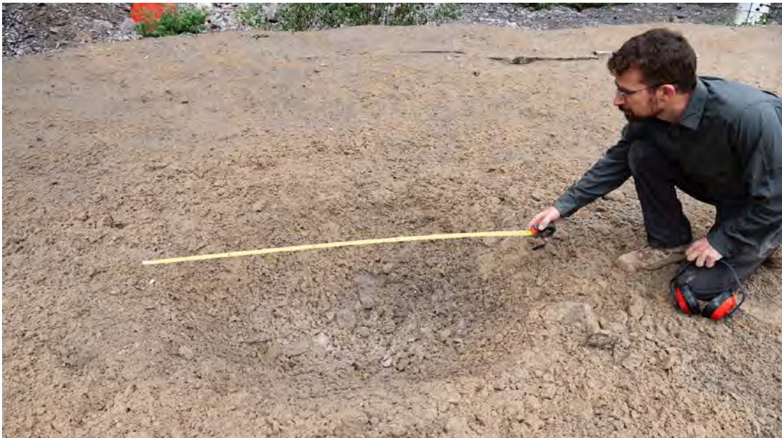
Image 5. The shaped charge has successfully penetrated the sand and achieved a high order explosion of the buried main charge
