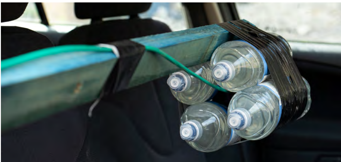
Image 2. MA IEDD operators often need to locally develop tools based on a sound understanding of explosive principles. Here an improvised disruptor has been constructed to cause general disruption of a vehicle-borne IED (VBIED)
