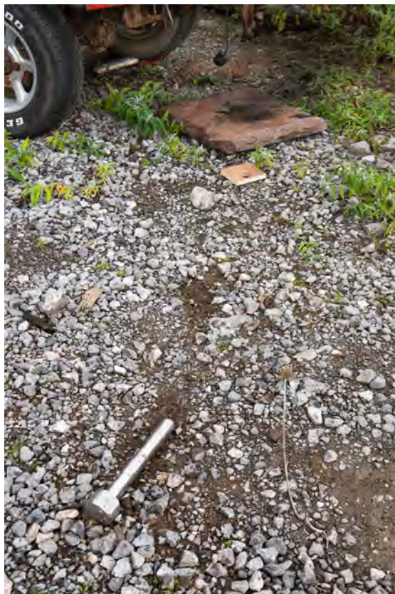
Image 8. The disruptor has successfully removed the power source from the suicide belt with the additional benefit of moving the belt from its original location. Note the disruptor recoil
