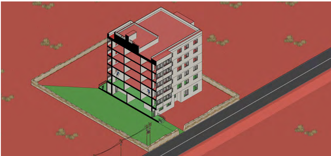
Image 4. Image showing a cutaway of a building portraying systematic recording: completed areas are annotated in green, areas to be searched remain in red
