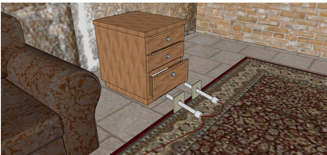
Image 1. Image of a double disruptor shot. Note the parallel placement of the barrels, wired in series
