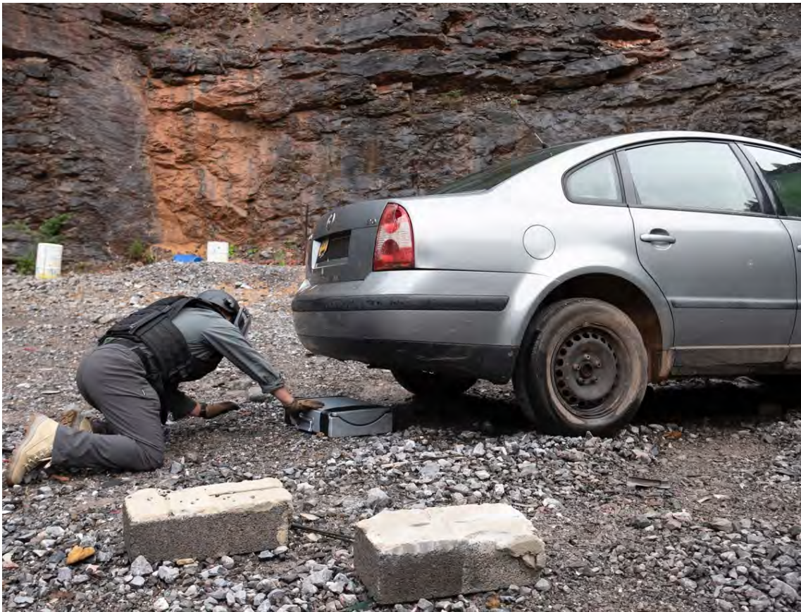
Image 29. MA IEDD operator manually placing VBIED extractor
