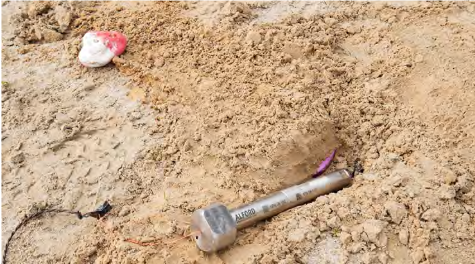
Image 4. Barrel disruptor targeting a buried power source uncovered during a fingertip search. The natural angle of the excavated channel has been used to place the barrel disruptor
