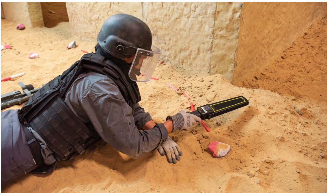
Image 10. Handheld detector used to delineate metal signature
