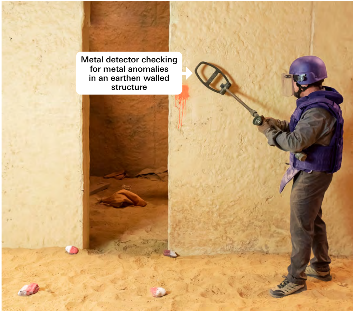
Image 7. Some buildings only contain limited metal in the structure yet metal detectors may still provide benefit to search operations
