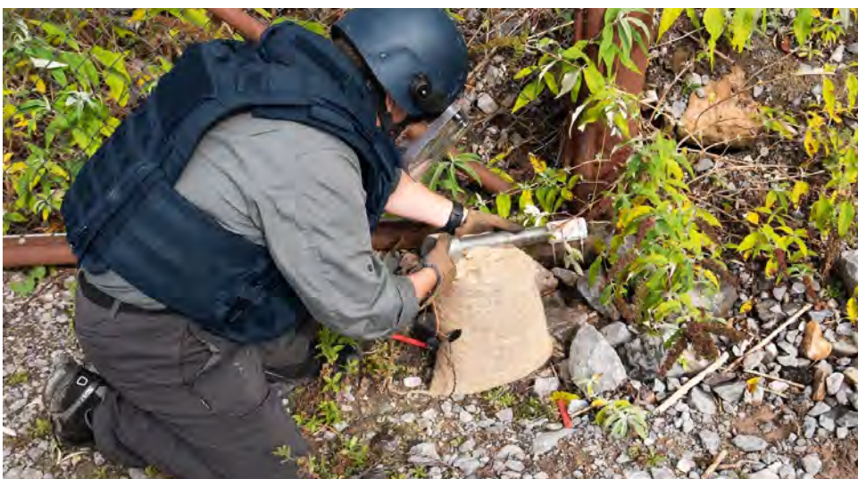
Image 6. An MA IEDD operator using a sandbag as an improvised stand to place a barrel disruptor targeting a legacy IED
