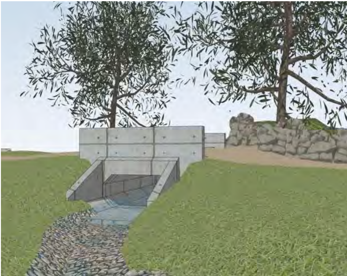
Image 23. Culverts provide an opportunity for the emplacement of IEDs
