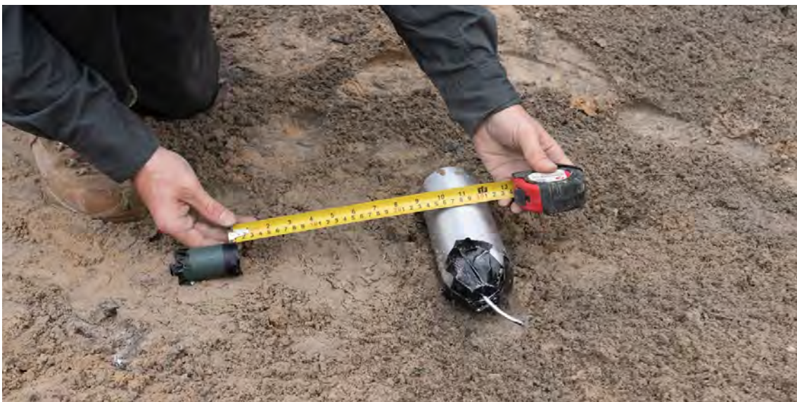
Image 13. Locally made shaped charge placed at 90 degrees to the centre line of the target with enough stand-off for the shaped charge to form
