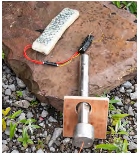
Image 5. Barrel disruptor targeting the power source on an abandoned suicide belt. A locally manufactured stand has been used to aid in correct placement
