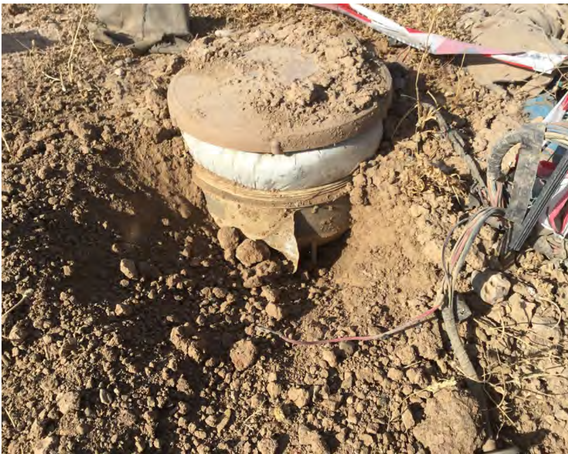
Image 12. VS-500 exhibiting expansion of the HME due to moisture as an effect of ageing (source: FSD ©)
