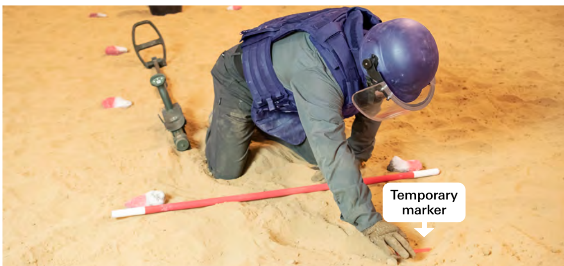
Image 7. Here a temporary marker is placed to indicate the centre mass of the suspect signal
