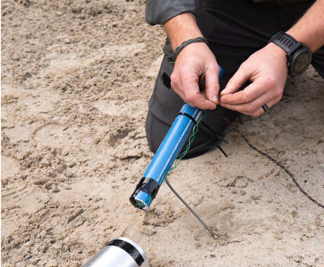
Image 2. Thermite lance placed to induce a burn in a thin metal cased main charge. Note how the lance has been placed at the rear to avoid the detonating cord
