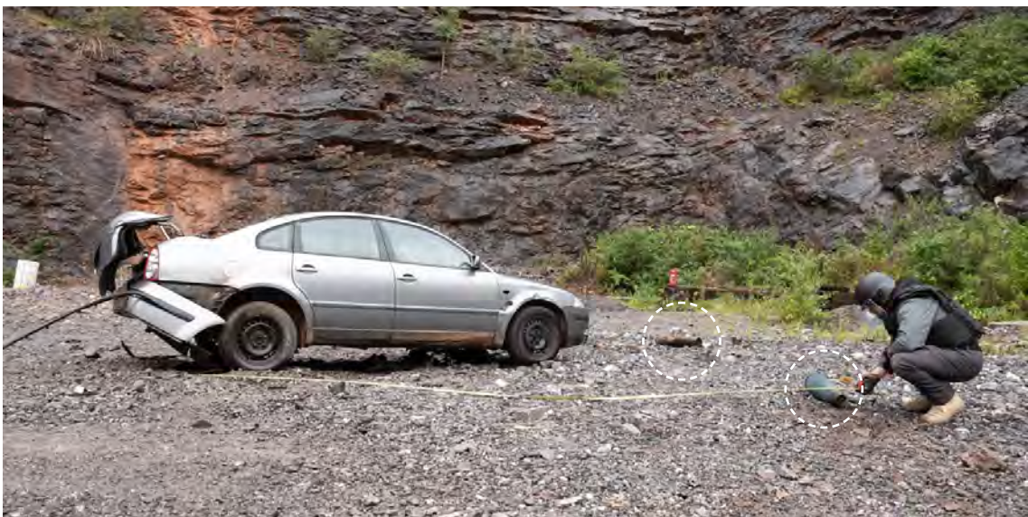
Image 38. Location of the two 155 mm projectiles post firing of the VBIED extractor
