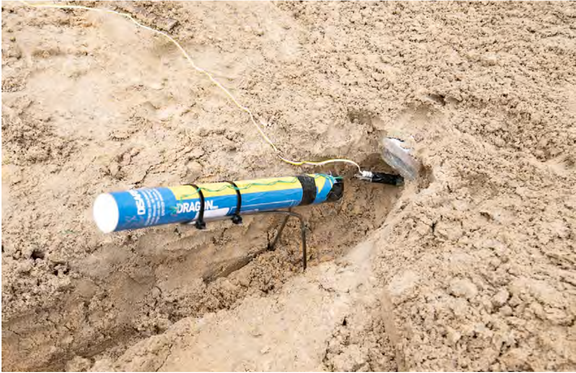
Image 3. Thermite lance placed to target the exposed detonator of an IED main charge
