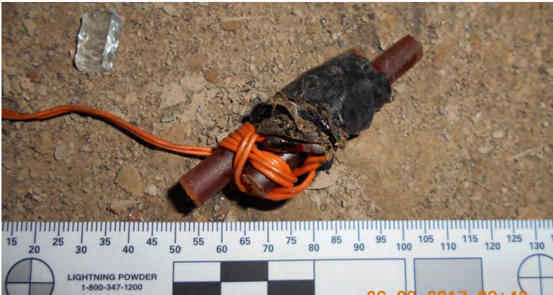
Image 190. Improvised rocket igniter (source: FSD ©)
