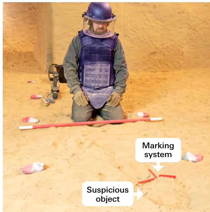
Image 3. An example of a clear marking system used to denote the location of a suspect object
