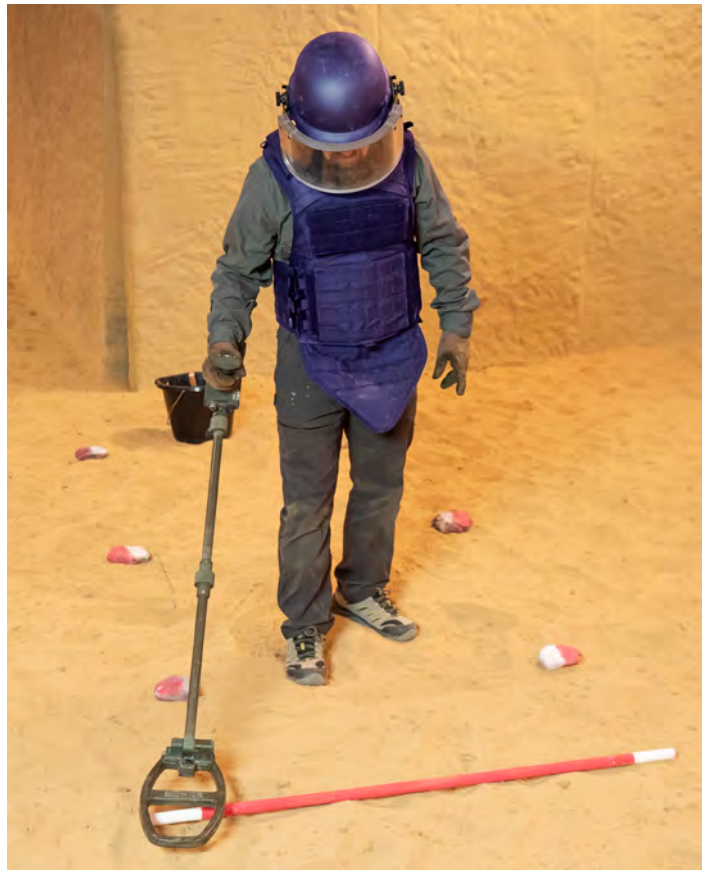
Image 5. Detector moving to the right-hand side. This is progressed with consistent overlap between sweeps within a comfortable forward limit for the searcher
