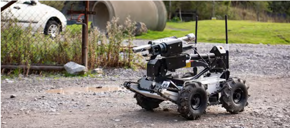
Image 1. Remotely operated vehicle (ROV) fitted with barrel disruptor, manipulator and wire cutter
