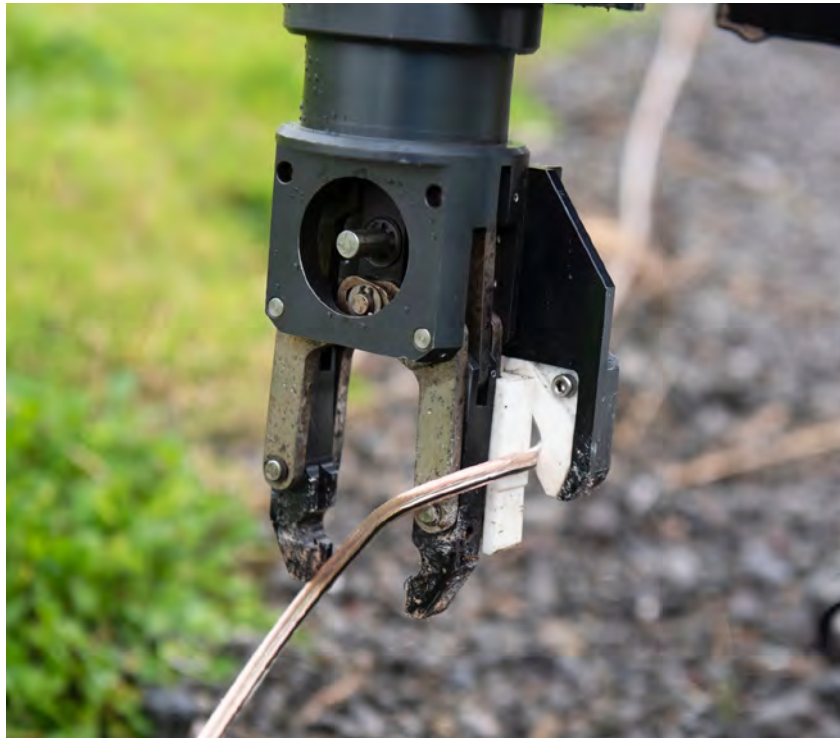
Image 4. ROV semi-remotely cutting an electrical link
