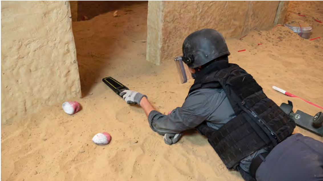
Image 17. A wand type metal detector is used, to more accurately delineate the subsurface components
