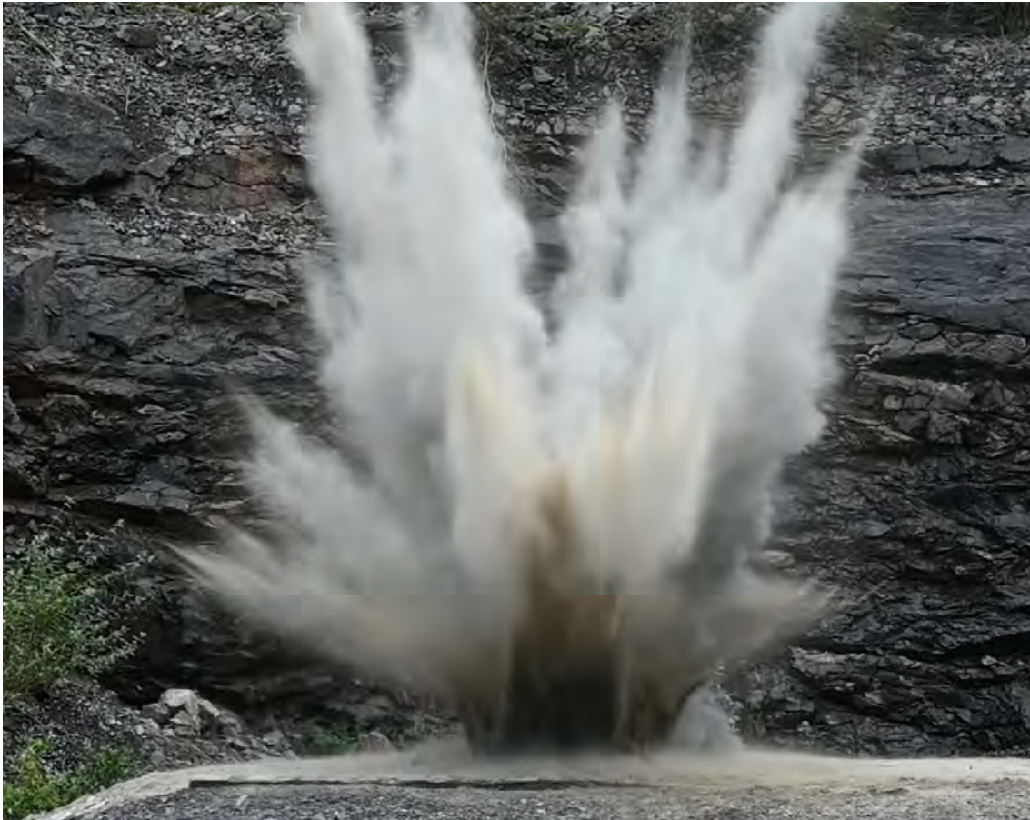
Image 1. 800 g of ANAL HME being destroyed in situ with a 100 g HE donor charge
