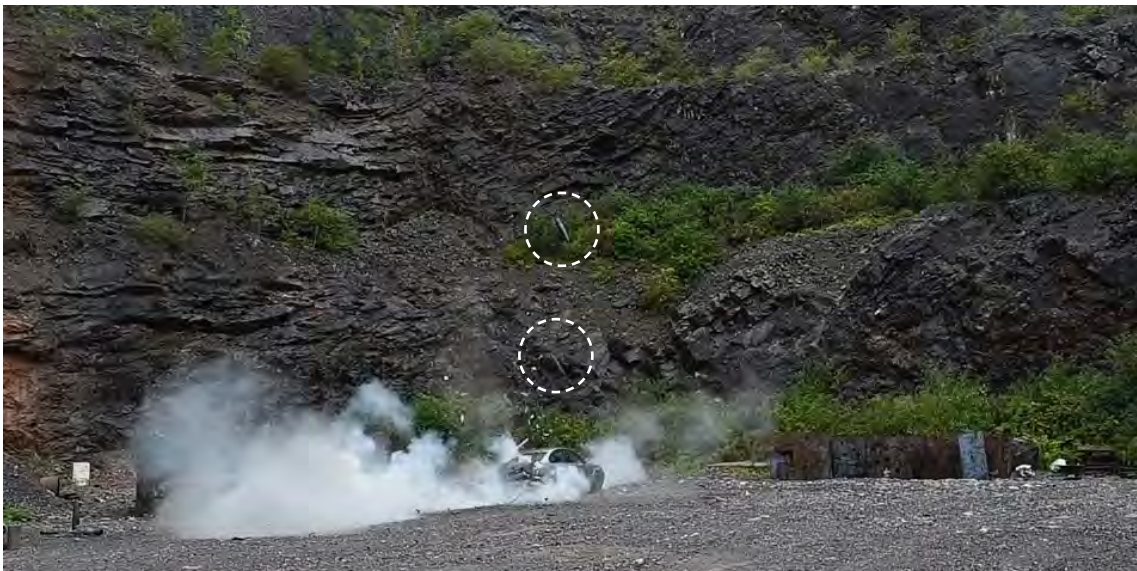
Image 34. Both projectiles have been extracted and are in the air above the vehicle
