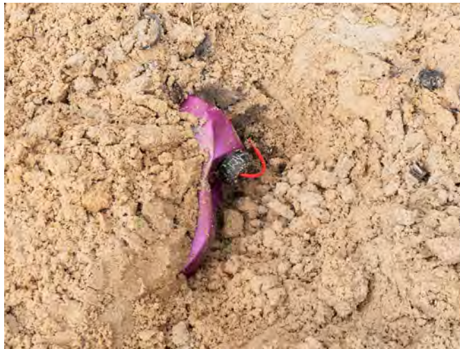
Image 7. The buried power source has been successfully removed from the circuit of a crush wire IED with minimal interaction by the IEDD operator
