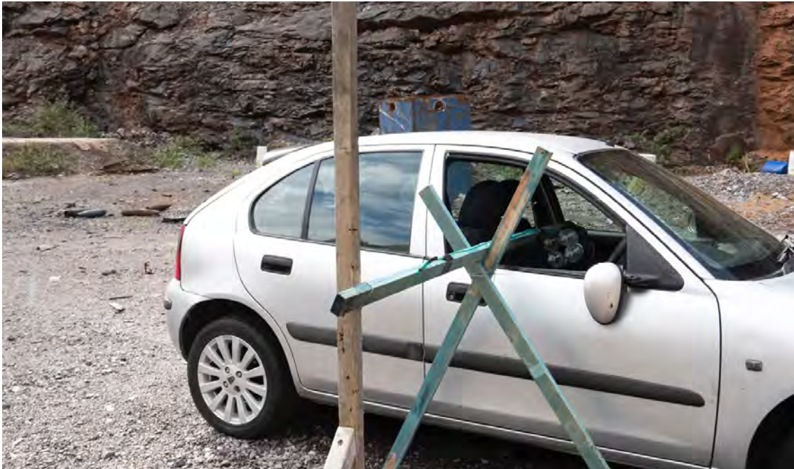
Image 18. Improvised stand used to place VBIED disruptor in the centre of the passenger area
