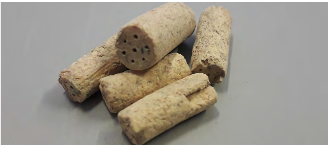
Image 20. Another example of propellant made of nitrocellulose. Drilling holes increases the surface of the prill and, therefore, the burning action. (source: Bundeswehr CBRN Defence Command ©)
