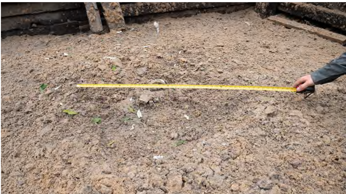
Image 9. Deflagration was unsuccessful and the main charge detonated. This highlights the difficulty in achieving deflagration of improvised main charges filled with HME of unknown provenance and unknown position of the detonating cord booster. However, the main charge has been successfully destroyed
