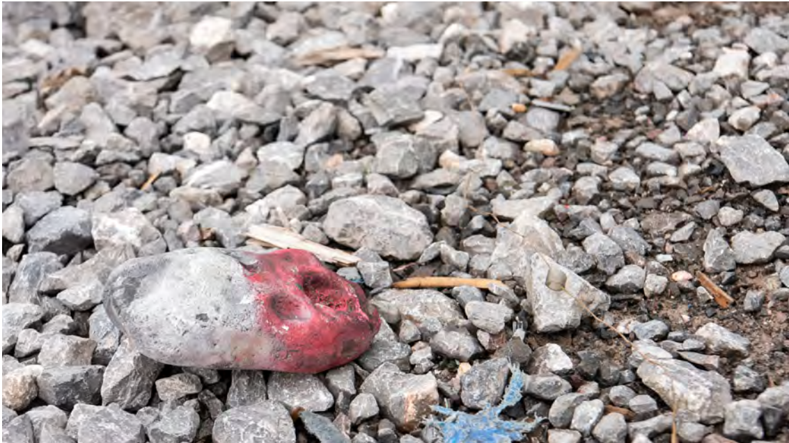
Image 40. A surface-laid pressure-activated switch
