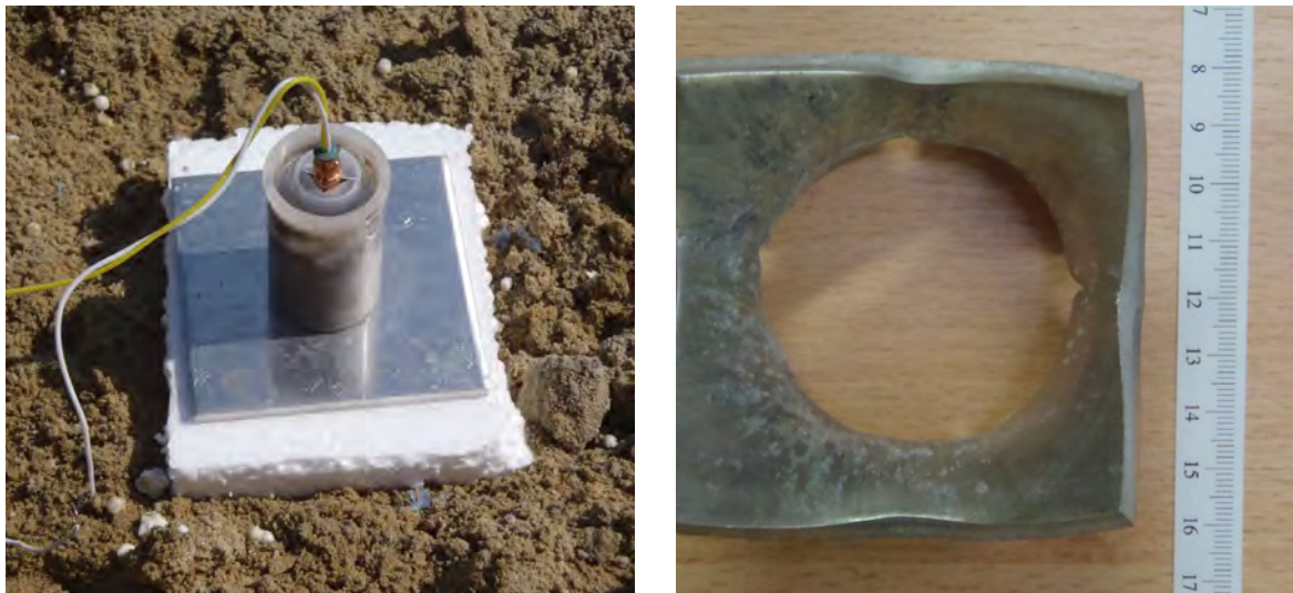
Image 165. Effects of a small quantity of home-made peroxide explosive on a metal witness plate (source: BCL ©)
