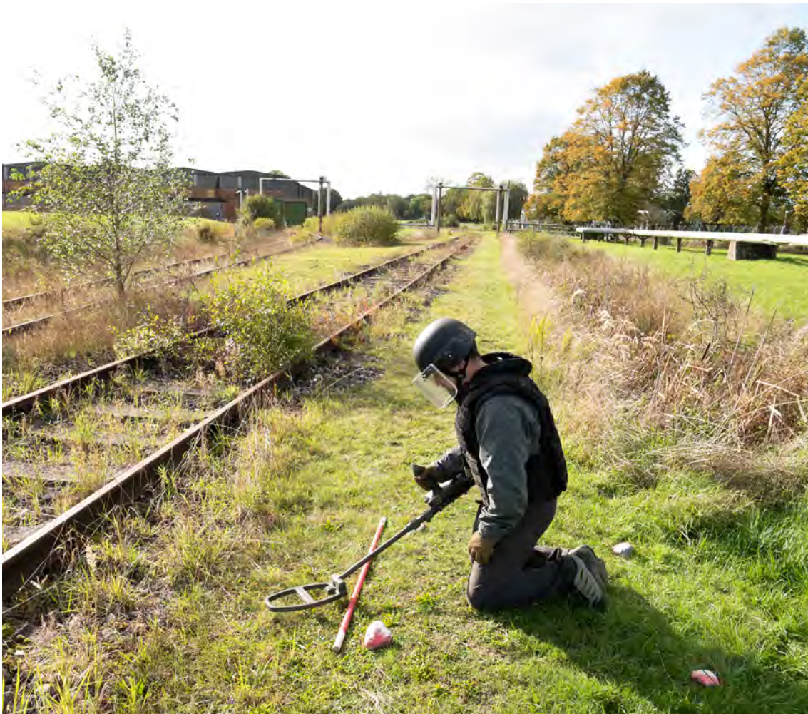
Image 3. In this example the threat of tripwires has been discounted and the searcher is only using a metal detector to search for subsurface IEDs
