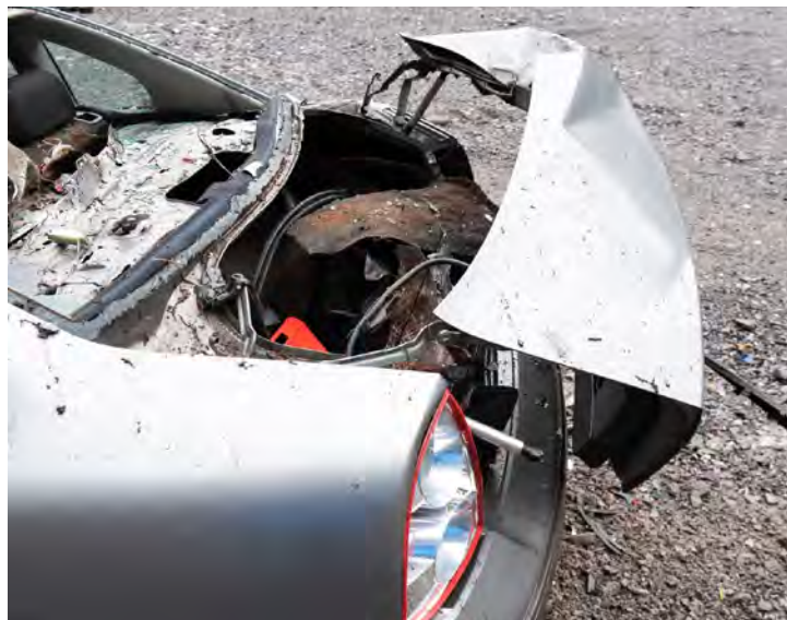
Image 35. Trunk post firing the VBIED extractor
