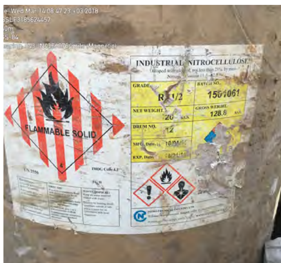
Image 107. Label on a drum used as a container for industrially produced nitrocellulose (source: FSD ©)
