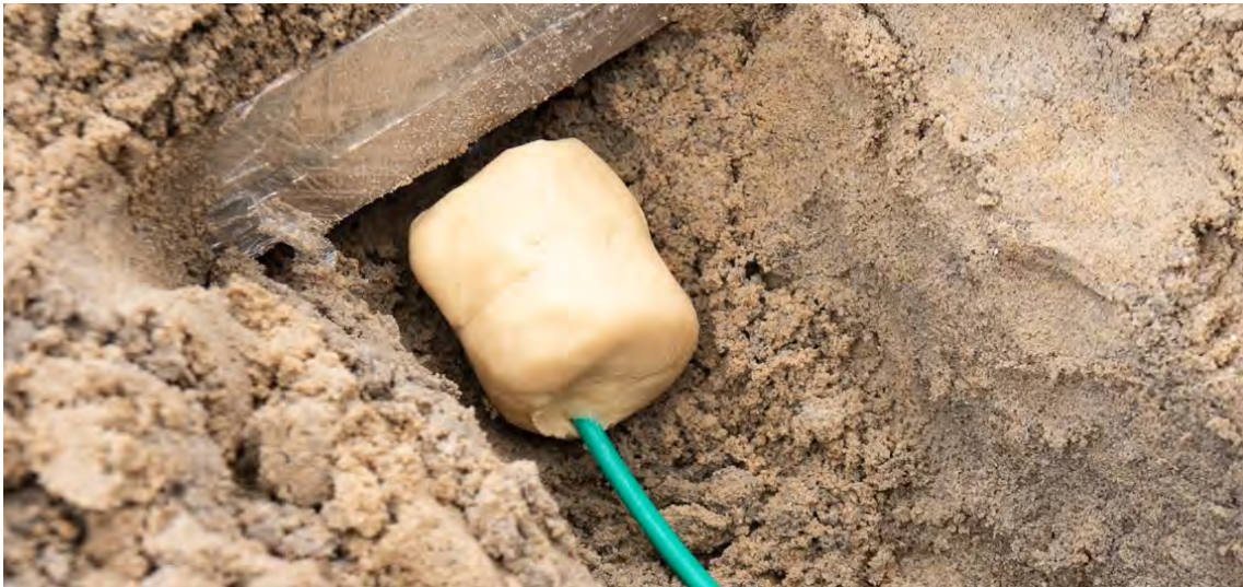
Image 5. Donor charge placed with increased stand-off
