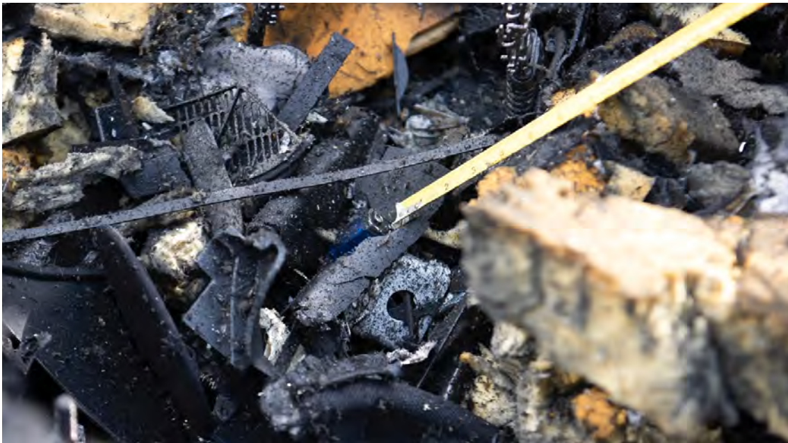
Image 26. Tape measure points to power source from RC pack. Remains of RC pack container can be seen below power source
