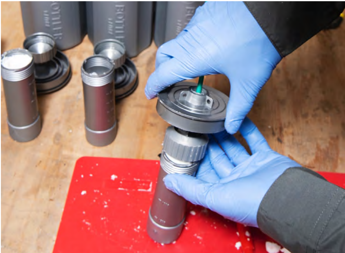
Image 2. Sealing the inner chamber of a commercial bottle disruptor
