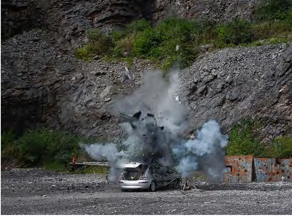
Image 1. Improvised VBIED disruptor firing on test range
