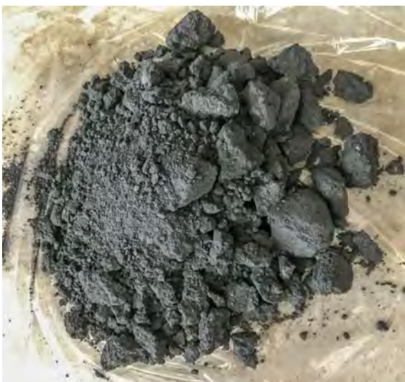
Image 174. Improved dynamite comprising nitroglycerine, potassium nitrate and charcoal (source: BCL ©)
