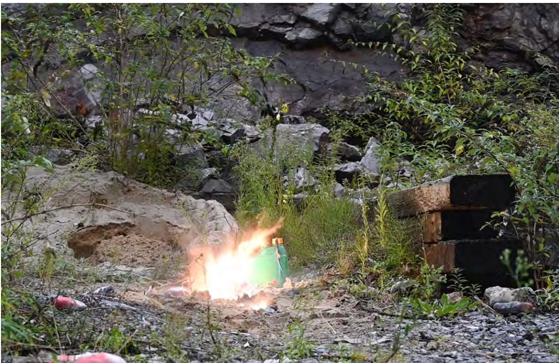
Image 17. The disruptor is functioned from the safety of the CP. Note the amount of heat and flash immediately on detonation
