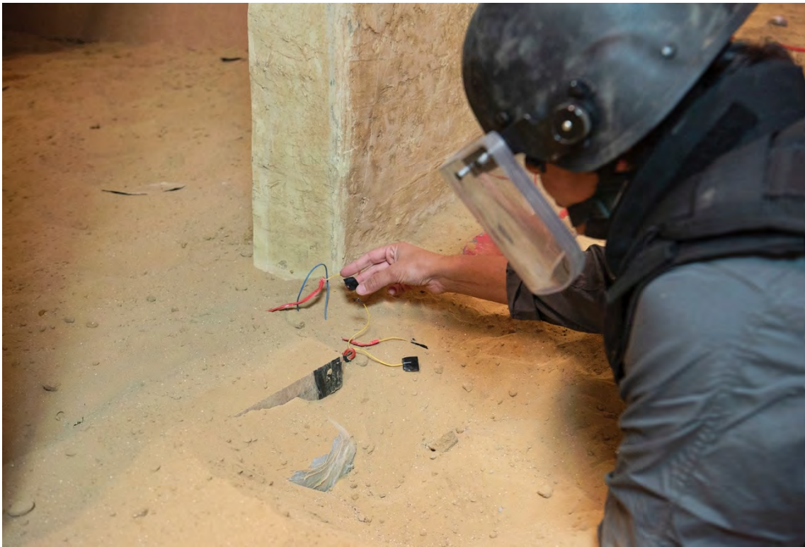
Image 23. Insulating second detonator lead
