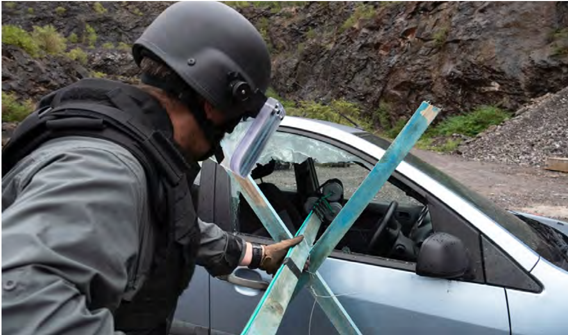
Image 8. Improvised stand being used to place VBIED disruptor in the centre of the passenger area
