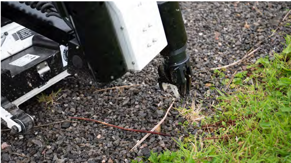
Image 3. ROV locating an electrical link
