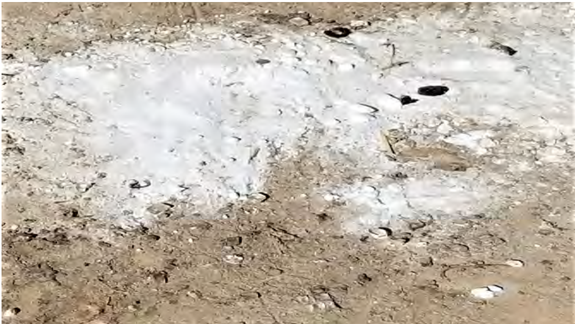
Image 202. Substance presenting a possible exposure to ammonium nitrate. Unprotected, the ammonium nitrate may be absorbed via breathing or via the skin. Ammonium nitrate dust stirred up by the wind can irritate eyes, mucous membranes or the respiratory system (source: GICHD ©)
