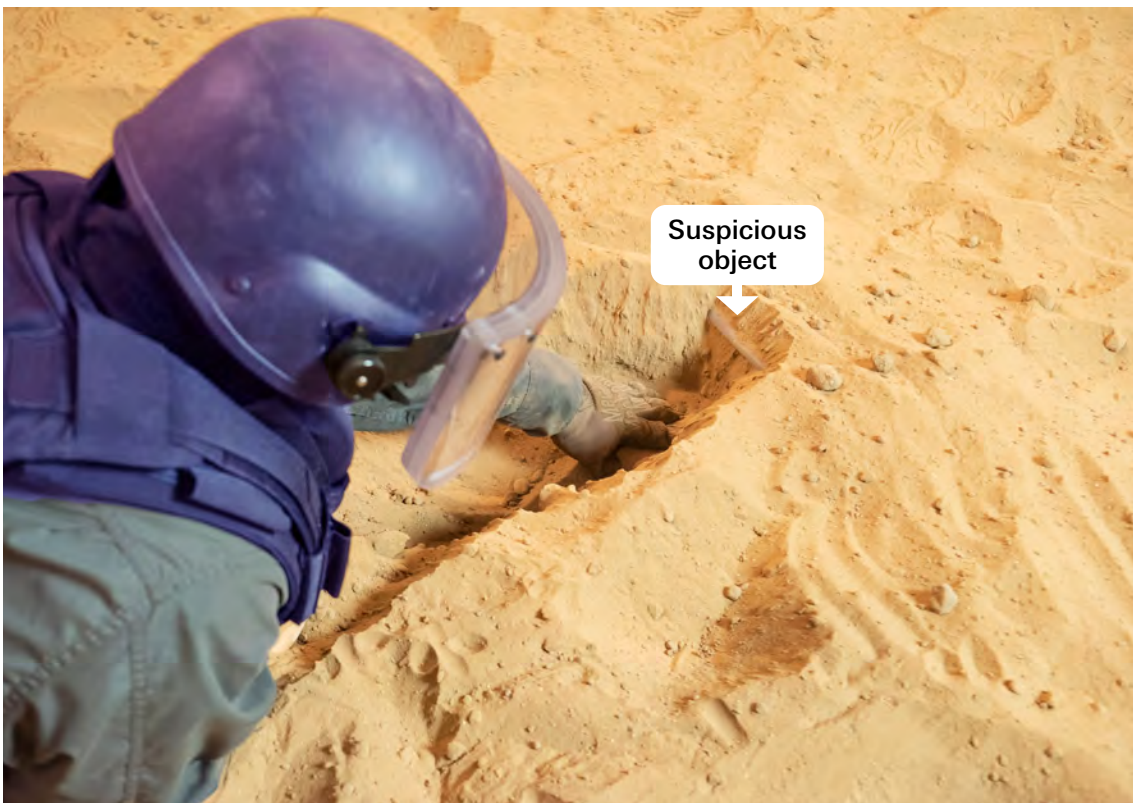
Image 12. A suspicious object has been located by excavation below it. At this point the searcher should make the assessment (dependent on accredited SOPs) on whether it has the potential to be part of an IED
