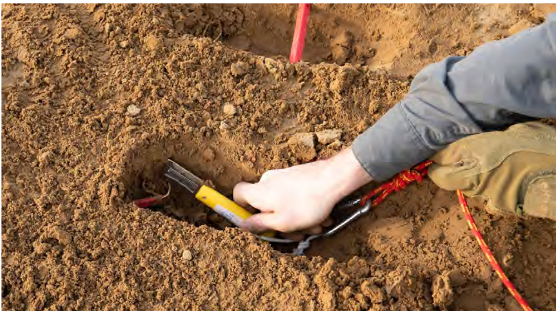
Image 3. Placing the cutter. Note how the IEDD operator is maintaining control throughout to prevent disturbance of the target wire
