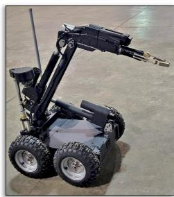
The R-BOT is a low-cost, unmanned ground vehicle (UGV) that can reduce or eliminate the time of danger for an operator who must inspect, x-ray, or disrupt a hazardous device.
