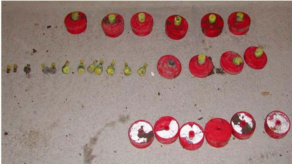
Figure 55. Examples of intact functional mines (top row), detonators separated from main charge (second row), and main charge separated from detonator (bottom row).
