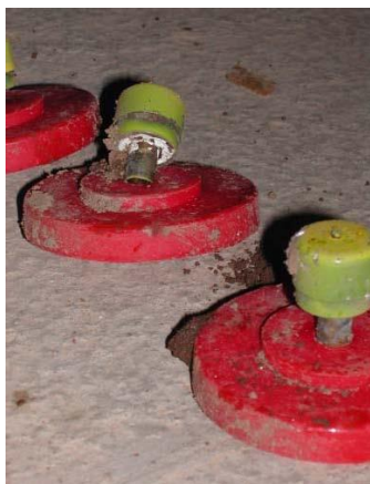
Figure 56. Detonators separated from main charge (left) and main charge separated from detonator (right).
