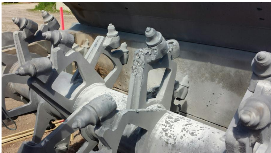
Figure 41. Results after detonation number 1. 5 kg AT-mine.
