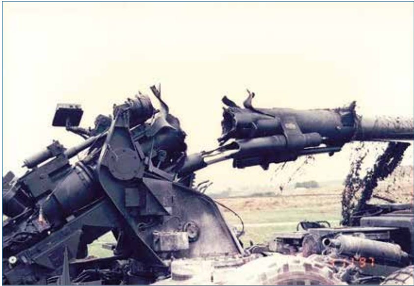
Figure 21 – Effects of a premature bore explosion on a Singapore Armed Forces 155 mm howitzer 271)
