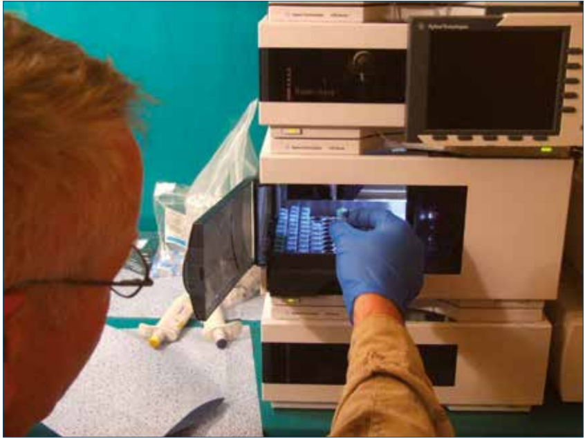
Figure 17 – Ammunition technician conducting propellant stabilizer assessment on ammunition 182)
