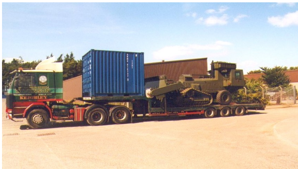
Figure 4 – Aardvark on a low bed trailer.
