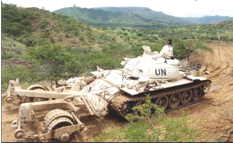
Figure 1 – T 55 tank roller operating in Eritrea
