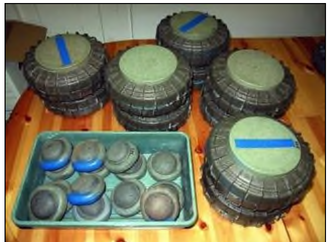
Figure 6: Inert SB-33 and SB-81 mines awaiting final safety checks and marking
