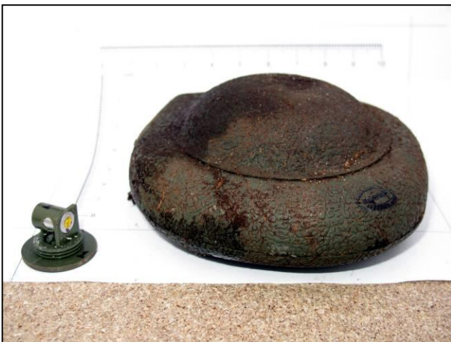
Figure 3: An SB-33 recovered from the Falklands; note the domed profile of the pressure plate
