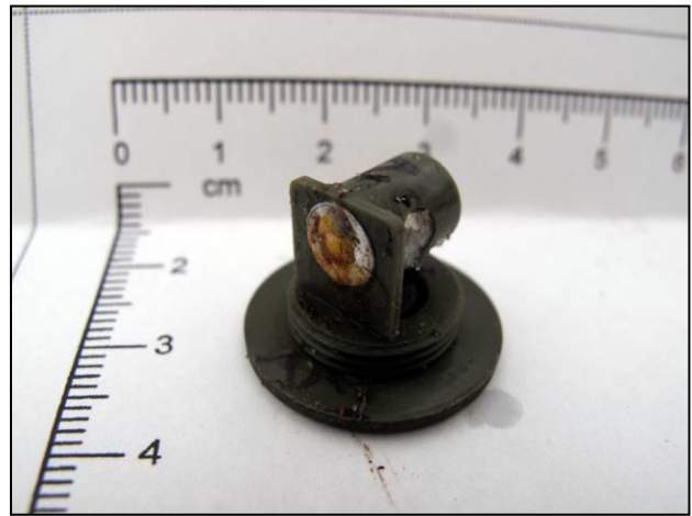
Figure 11: The yellow seal on the stab receptor appears to have been breached
