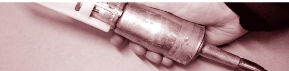
Illustration 4 | Sous-munition antiblindé Rockeye | © Colin King
