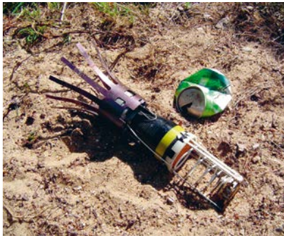
16 The British BL 755 is initiated by a nose-mounted piezo-electric element. The fuze incorporates both mechanical and electrical safety features
