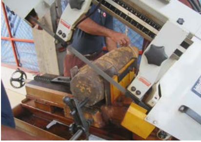
25 A projectile is cut open to gain access to the explosive
