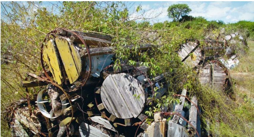
23 These cluster bombs in Mozambique have been stored outside for many years, deteriorating as a result of exposure to high temperatures and rain
