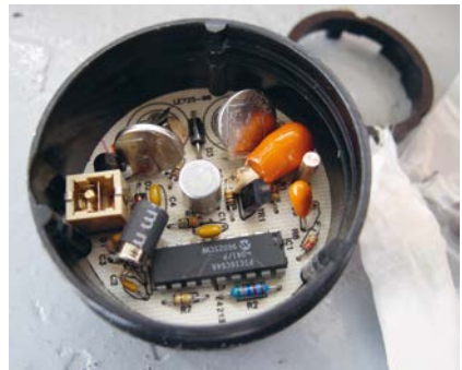
20 The electronic fuze of the Spanish SNA submunition. Circuits like this are less prone to malfunction than mechanical systems, and each one can be tested prior to production
