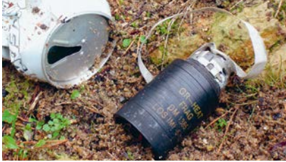
19 The Israeli M85 incorporates a self-destruct mechanism, but this has proven far less reliable than claimed
