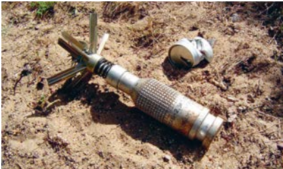
11 The Russian PTAB-2.5KO is a dual-purpose submunition, combining a HEAT shaped charge with a notched fragmentation casing
