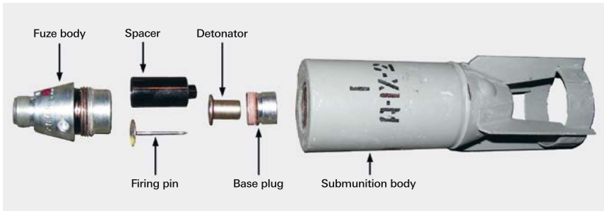
17 Components of the Russian AO-1Sch. The fuze has no safety or arming mechanism; sufficient impact simply crushes the nose of the fuze and drives the firing pin into the detonator
