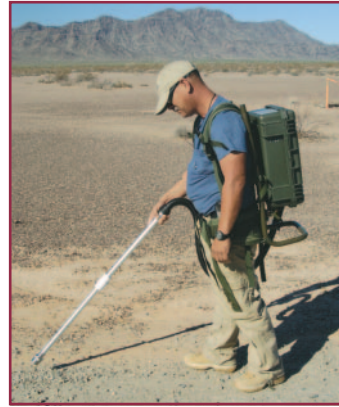
Figure 3. High-volume sampling in a test minefield using a Nomadics battery-powered pump.
