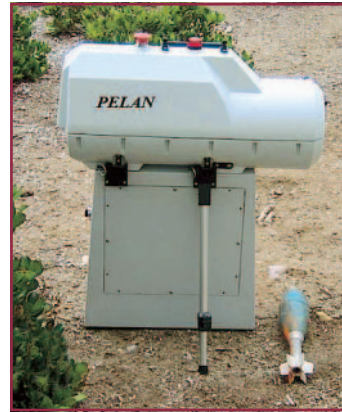
Figure 1. A complete PELAN unit.
