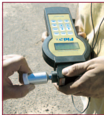
Figure 2. Analysing a high-volume sample collection filter using the Fido X.
