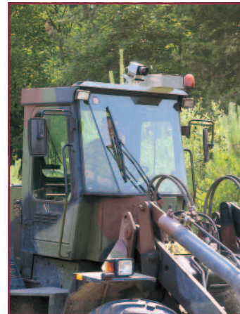
Figure 2. The polarisation camera mounted on the wheel loader. The metal box right of the camera contains the computer.
