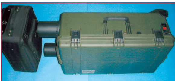
Figure 1. The SENNA portable device for detection of concealed explosives, here inspecting a suitcase.
