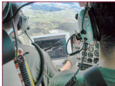
Figure 2. The pilot and co-pilot see the real time position of the helicopter on the large screen, while the background can be a map, ortho photomap or geocoded satellite image. On the map an area of interest is displayed, together with the planned and realised flight routes.
