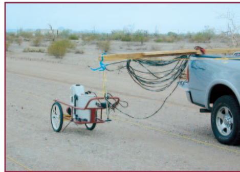
Figure 2. The PELAN evaluated in the US as an anti-personnel mine identifier (2003).
