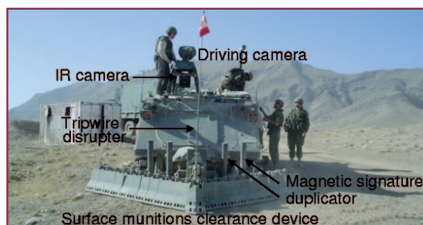
Figure 2. The ILDS protection vehicle (PV), which precedes the RDV and removes anti-personnel mines and some types of anti-tank mines such as magnetic influence and tilt-rod activated mines prior to the RDV searching for the remaining anti-tank mines.
