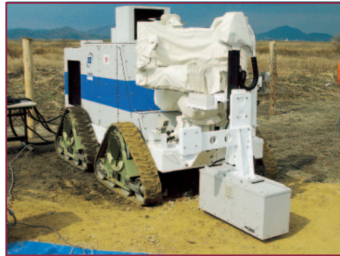
Figure 1: LAMDAR-III mounted on the front of the Mine Hunter Vehicle.
