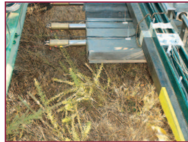
Figure 2. Close-up of XMIS detectors and location on test lane where the 5cm DOB TS 50 AP mine was located.
