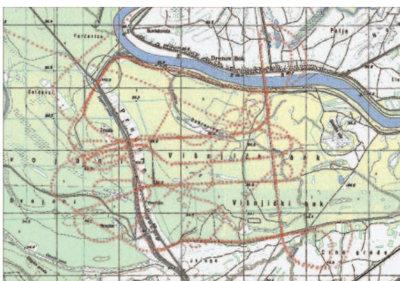
Figure 3. A view of the flight route on the topographic map at the scale 1:25,000. This serves as an example of the aerial survey of the electricity high voltage network (state of the towers, vegetation) and access field roads from the asphalt road on the left side of the network corridor.
