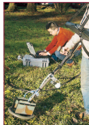
Figure 1. ALIS and details of the search head.
