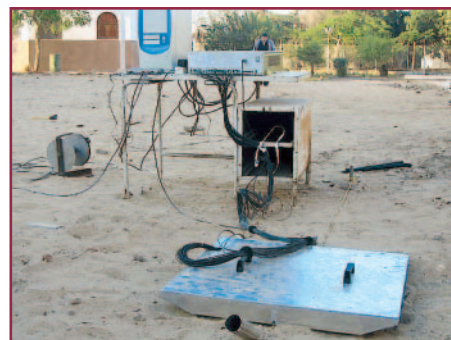
Figure 2. The DUNBID detector positioned on the sand during tests in Egypt. The position calculation electronics and the PC for data acquisition and measurement control are placed on the table.
