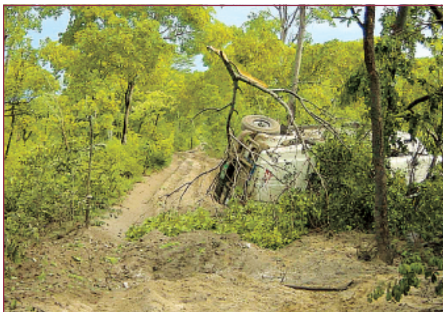
Figure 2. The blast of an anti-vehicle mine detonation can throw a vehicle up in the air. Such violent motions are one of the primary causes of deaths and injuries.
