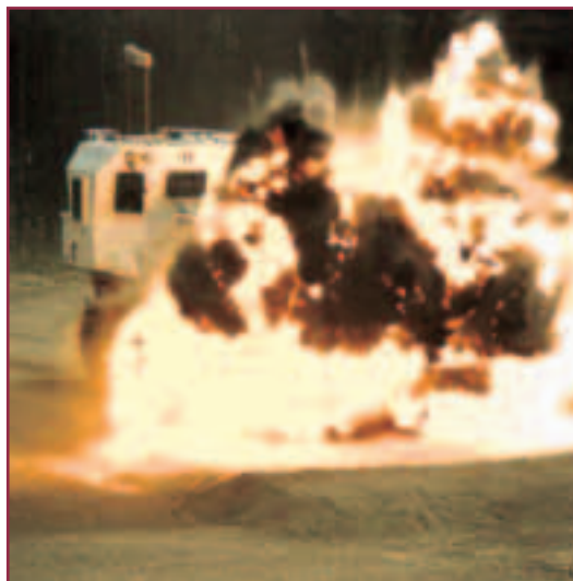
Figure 5. The power of anti-tank mine detonations is too great for most mechanical clearance systems to withstand without substantial damage. Mineguzzler. © Bofors.
