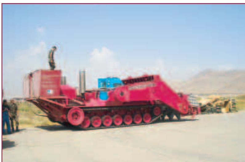
Figure 6. Systems that can withstand MOTAPM detonations are often too difficult to operate in post-conflict environments. Minebreaker 2000/2. © FFG.
