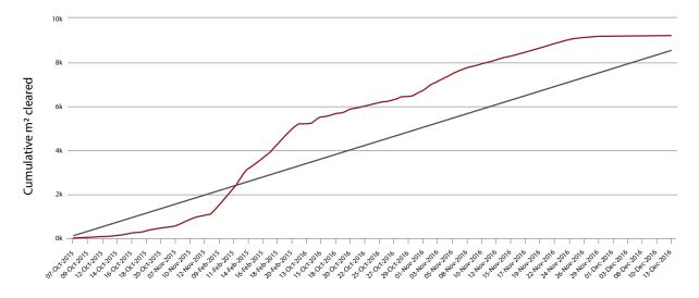
Figure 6. Progress chart showing a period when the production rate fell below the target line, followed by the deployment of additional clearance assets to increase the production rate and final completion around the target date. *Figure courtesy of Fenix Insight Ltd.*
