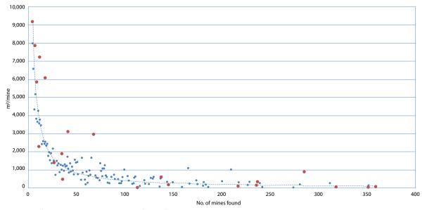
Figure 2. M<sup>2</sup>/mine data from Tajikistan (in red) showing the generally close alignment with the data from Afghanistan (in blue): Survey Action Center Tajikistan Land Release Project Report 2011. Base data was provided by MACCA and the Tajikistan National Mine Action Centre (TNMAC). *Figure courtesy of David Hewitson.*
