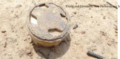
An M-14 minimum-metal, anti-personnel mine from a site where the vegetation was removed through burning. Comparisons of m<sup>2</sup>/deminer/dour, m<sup>2</sup>/searcher/day, or mines found/day must take into account the nature of EO found in order to be valid. *Image courtesy of Roly Evans.*
