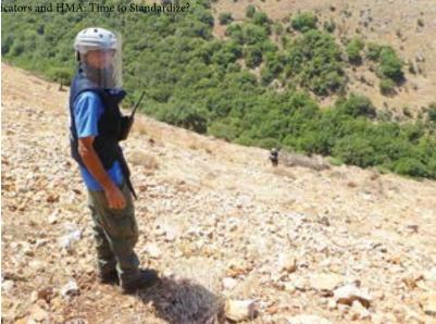
Metal contamination is one of the key factors affecting  $m^2$ /searcher/day. The image above shows an area where the battle area clearance (BAC) searcher has excavated many times for each  $m^2$  in the search for explosive submunitions.
