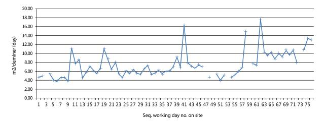
Figure 3. M<sup>2</sup> productivity/deminer, ratioed to a standard six-hour day equivalent (to ensure like-for-like comparability). A general upward trend in the KPI indicates deminers becoming familiar with site conditions. Stand out peaks in productivity were associated with areas where adjacent mines were blown in situ, breaking up nearby soil and vegetation, making it much easier for deminers to progress. *Figure courtesy of Fenix Insight Ltd.*
