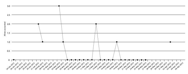
Figure 5. Mines found/day, an irregular profile associated with a mined area that is harder to "unlock." *Figure courtesy of Fenix Insight Ltd.*
