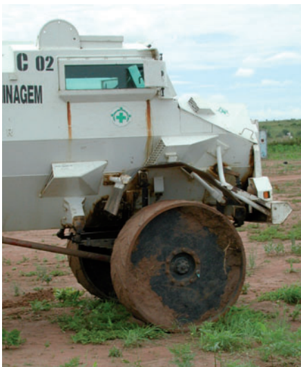
Casspir mine-protected vehicle with steel wheels
