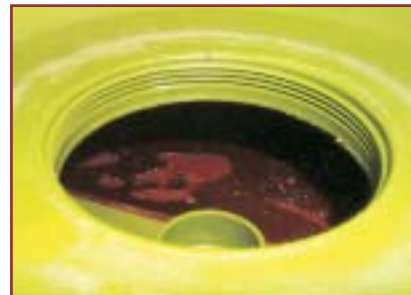
Figure 5 Coating on TMA-5 main charge explosive
