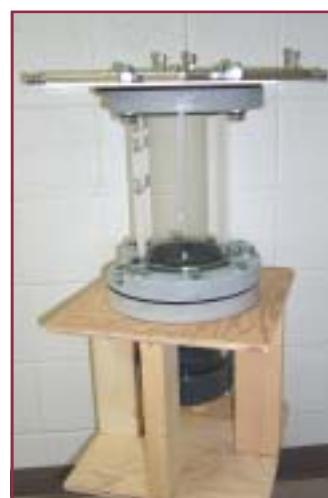
Figure 29 Laboratory soil column test apparatus
