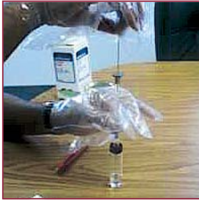
Extracting tripwire vapour.
