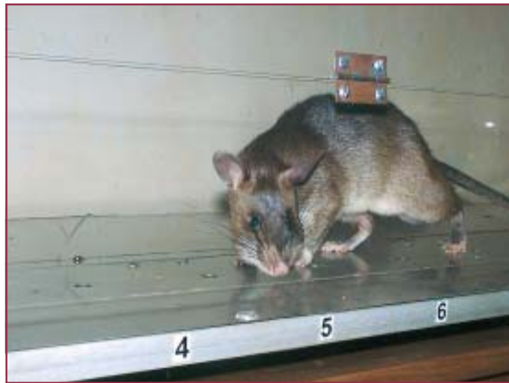
Rat analysing REST filters (the filters are placed below the walking track).
