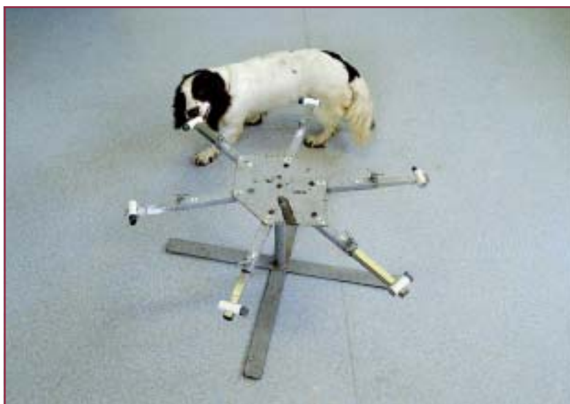
The multiple-choice training apparatus with Hindi checking a filter. As training progressed, the number of arms on the apparatus was increased to 12.
