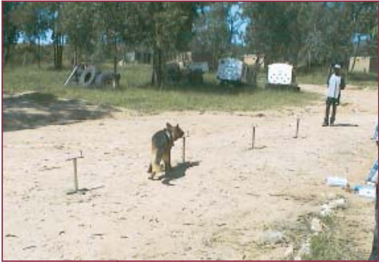
Search of filter cartridges mounted on six stands in a row (NPA, Angola).
