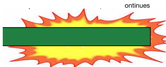
Figure 5: A weapon functioning as designed. In each step the energy delivered (green) exceeds the energy demanded (red) by the next step.
