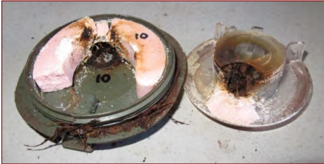
Figure 7: A disassembled Italian SB33 anti-personnel landmine showing the results of an age-weakened detonator that functioned, but failed to initiate the main charge.
