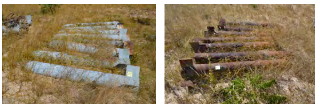
Figure 2: Weapons of the same type (Russian S24 air launched ground attack rockets) and age, from the same stockpile. The weapons on the right appear to have been subject to high temperatures, perhaps during a bush fire. The risk implications of the apparently different histories on the two groups of weapons are uncertain. Note that these weapons are not abandoned (AXO), but are in a stockpile under (limited) management.
