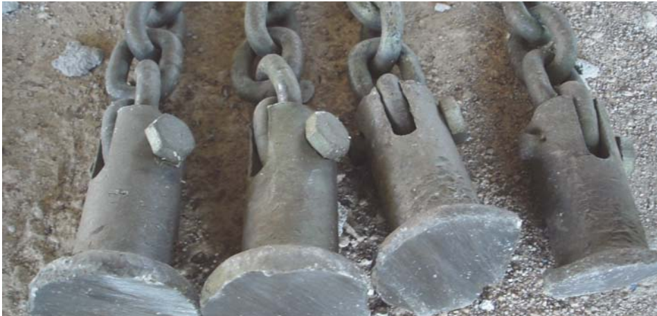
A chisel hammer (tungsten coated)
