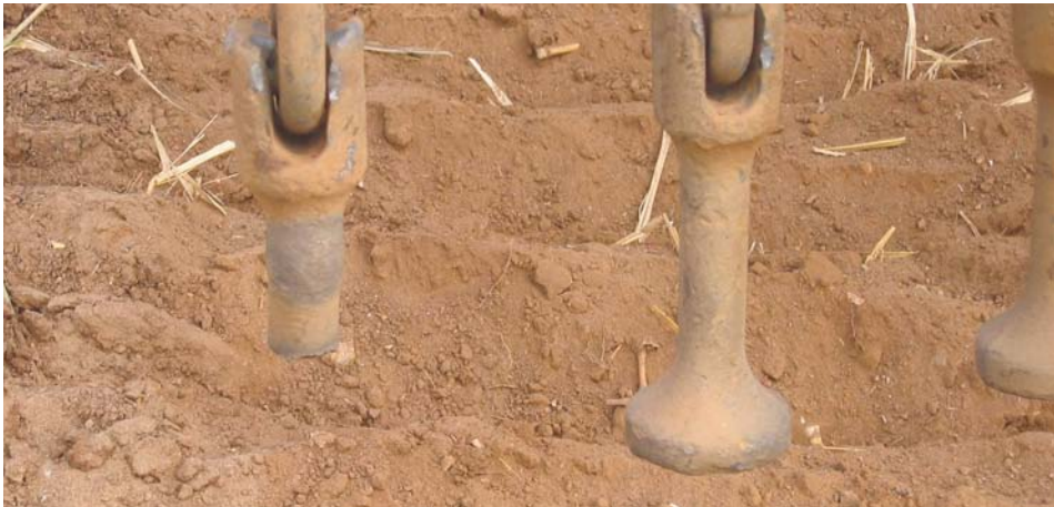
A broken hammer head after use in Sudan
