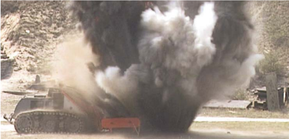
A Bozena 5 detonating an AVM mine (9kg TNT)
