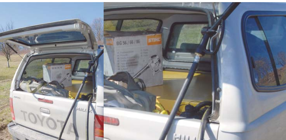
A mobile refuelling system: a pick-up fitted with a fuel tank
