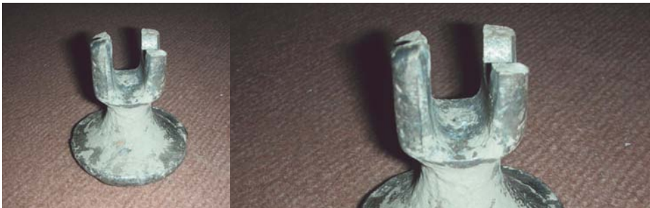
A broken hammer head after use in Afghanistan
