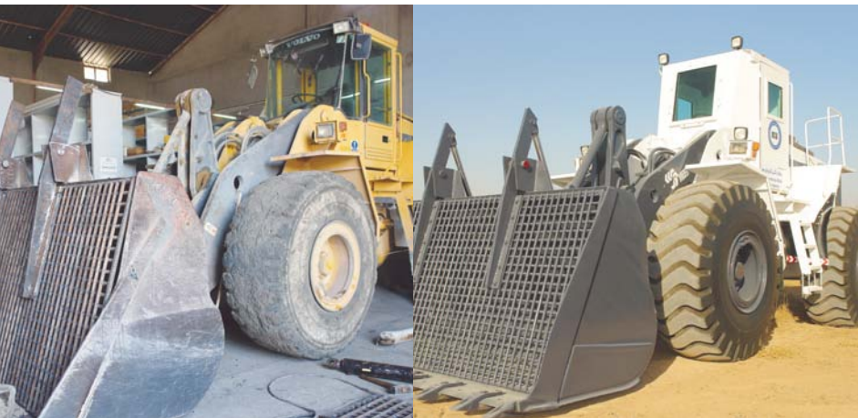
BEFORE | A front-end loader in Kurdistan being converted to a demining machine AFTER | The same machine as an armoured front-end loader with sifter
