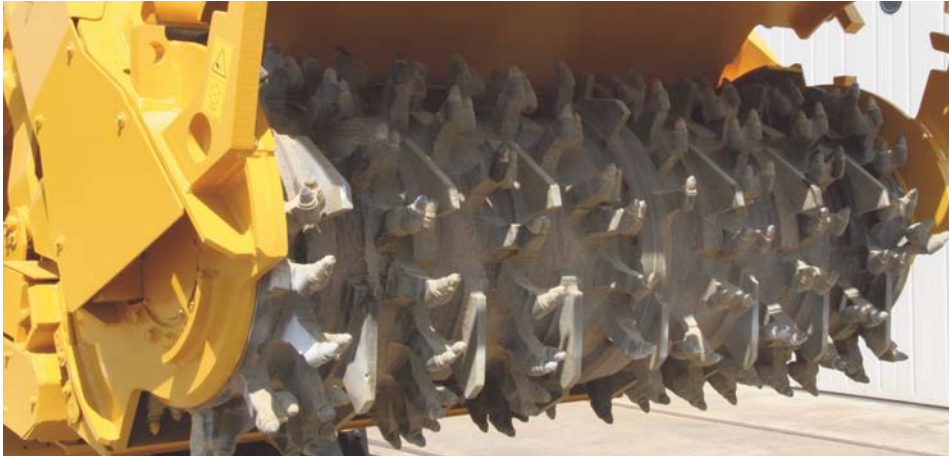
A counter-clockwise chisel tiller design
