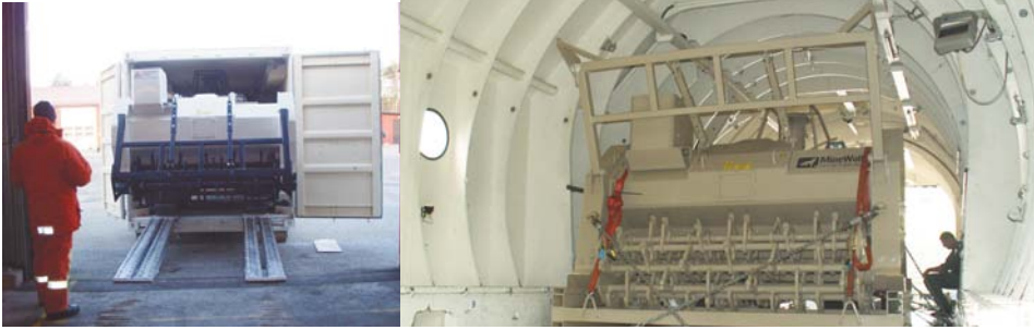
Loading a Mini MineWolf into a sea container | A Mini MineWolf loaded onto an aircraft
