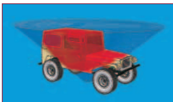
Fig. 11. The effect of the cone of destruction on a light, unprotected vehicle from a centre blast underneath the hull
