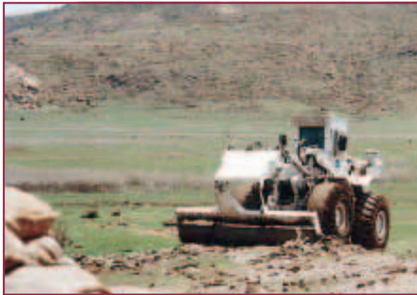
Fig. 25. Armoured Terex front-end loader with Pearson roller. Eritrea - Ethiopia border, 2001.
