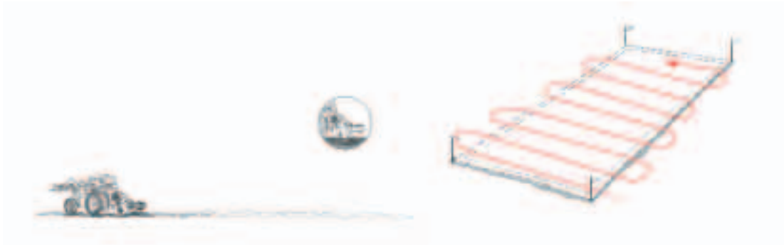
Fig. 22. The magnet follows the same pattern as the heavy cultivator collecting metal fragments or mines.
