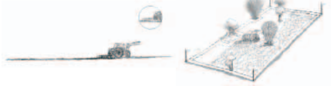
Fig. 19. Light cultivator is the first step in sub-surface investigation for evidence of mines.
