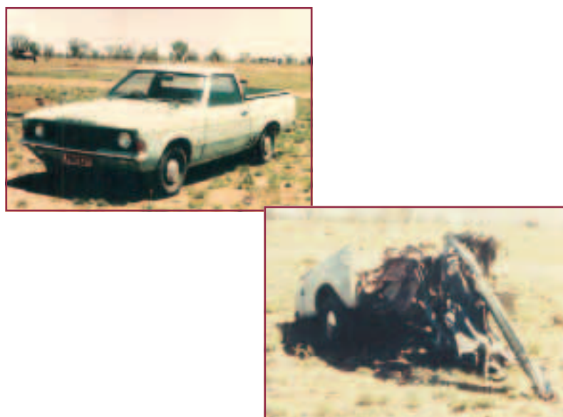
Fig. 12. The effect of a single TM-46 anti-tank blast mine detonated underneath the centre of an unprotected light vehicle
