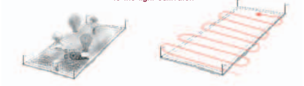
Fig. 21. The heavy cultivator is pulled in a different direction to the light cultivator.
