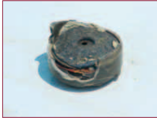
Fig. 11. M14 anti-personnel blast mine after a flail had passed over it in Lebanon. The firing pin is missing. What is required to initiate this mine now? What form of follow-up is now required to the area it was in; mechanical, manual or dogs?
