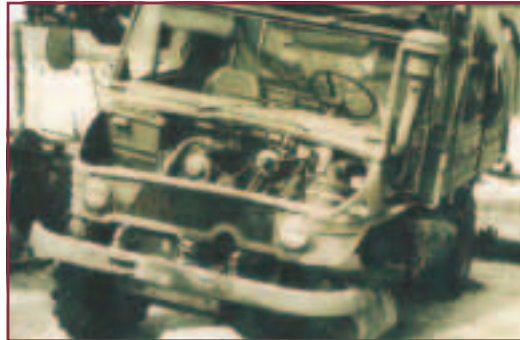
Fig. 22. Unimog vehicle fitted with protection plates in wheel area and wheels filled with water
