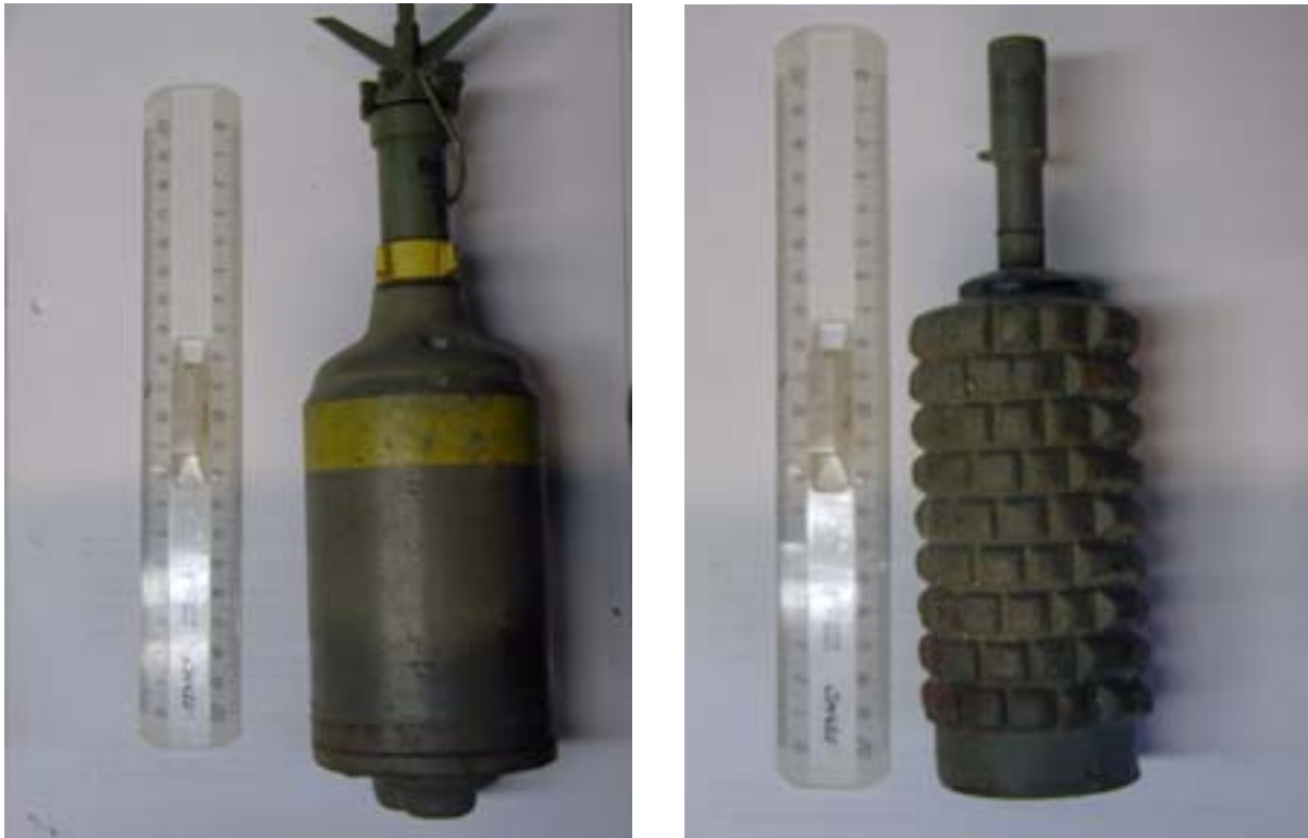
Figure 5.36: Metallic mines. Left: PROM (bounding fragmentation), Right: PMR-2A (stake fragmentation; stake not shown). Origin: Ex-Yugoslavia. Ruler length: 20+2.5 cm.
