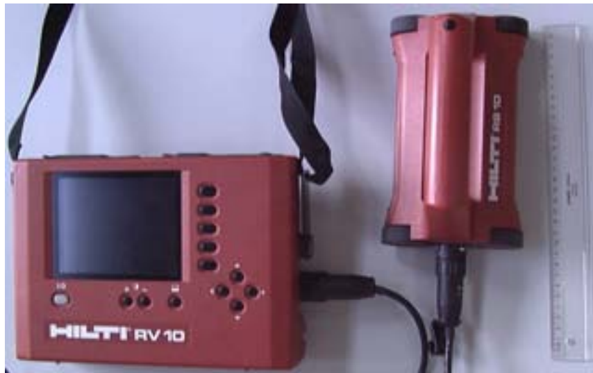
Figure 7.5: Ferroskan RV 10 monitor (left) and RS 10 scanner (right) (ruler length: 30 cm)
