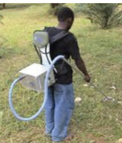
FIGURE 4 | Electric sampling pump developed by APOPO.
