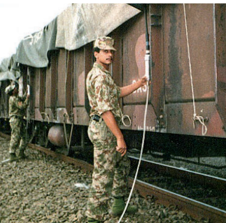
REST (MEDDS) used to detect traces from weapons in cargo in South Africa (mid-80s)
