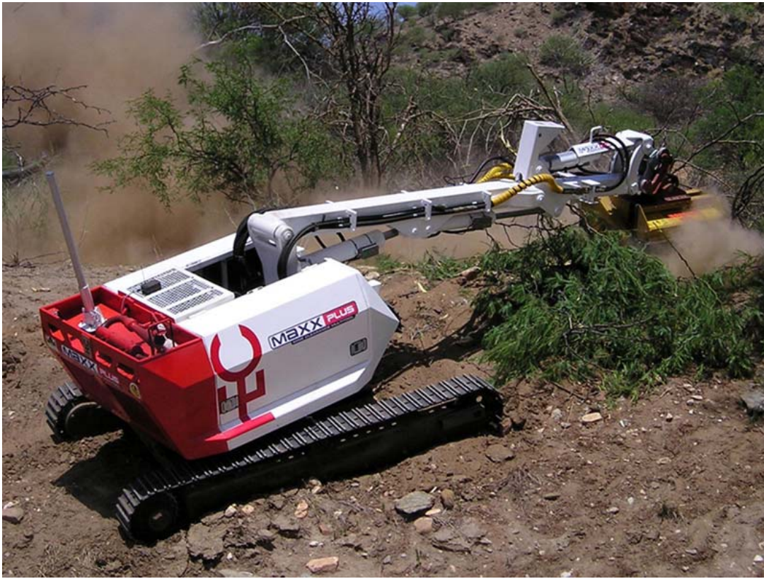
4. The MAXX v2 machine with mulcher attachment.
