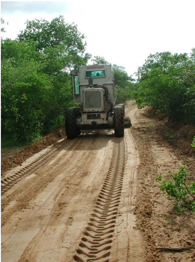
2. A motor grader used in the Voodoo System.
