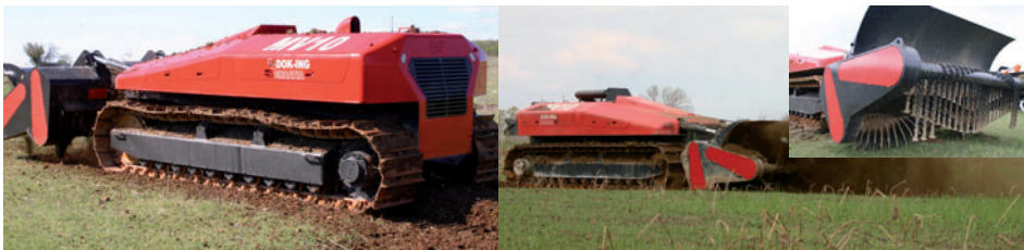
An example of a combined tiller and flail system | the MV10
