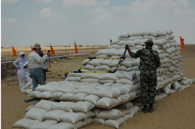
A semi-permanent ramp for testing a number of detectors on a variation of targets.
