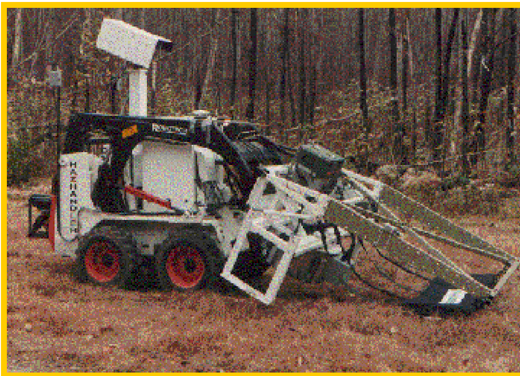
26. The NVESD prototype version mounted to a skid-steer.
