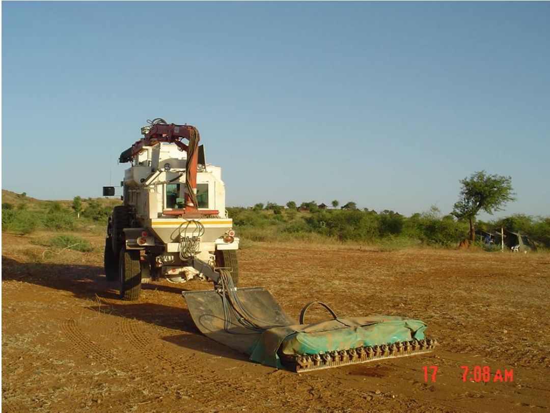
29. VAMIDS mounted on a mine-protected vehicle, in service with MECHEM.
