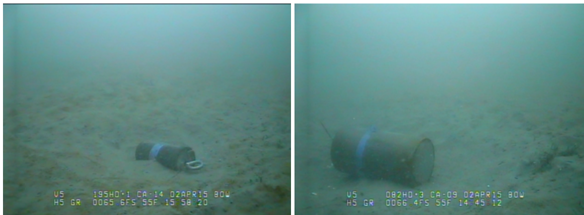
Figure 15. Screen captures of simulated ERW targets used in the technology demonstration. On the left, a two-inch diameter target; on the right, a six-inch diameter target.
