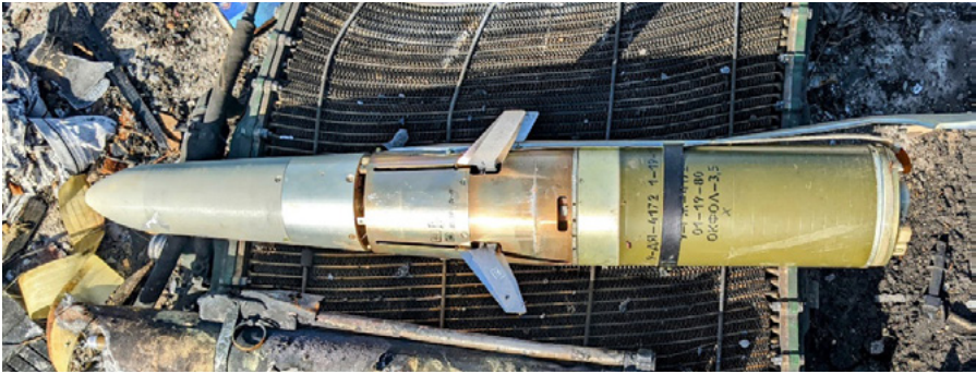
AT-16 missile warhead and guidance section. © Sean Moorhouse
